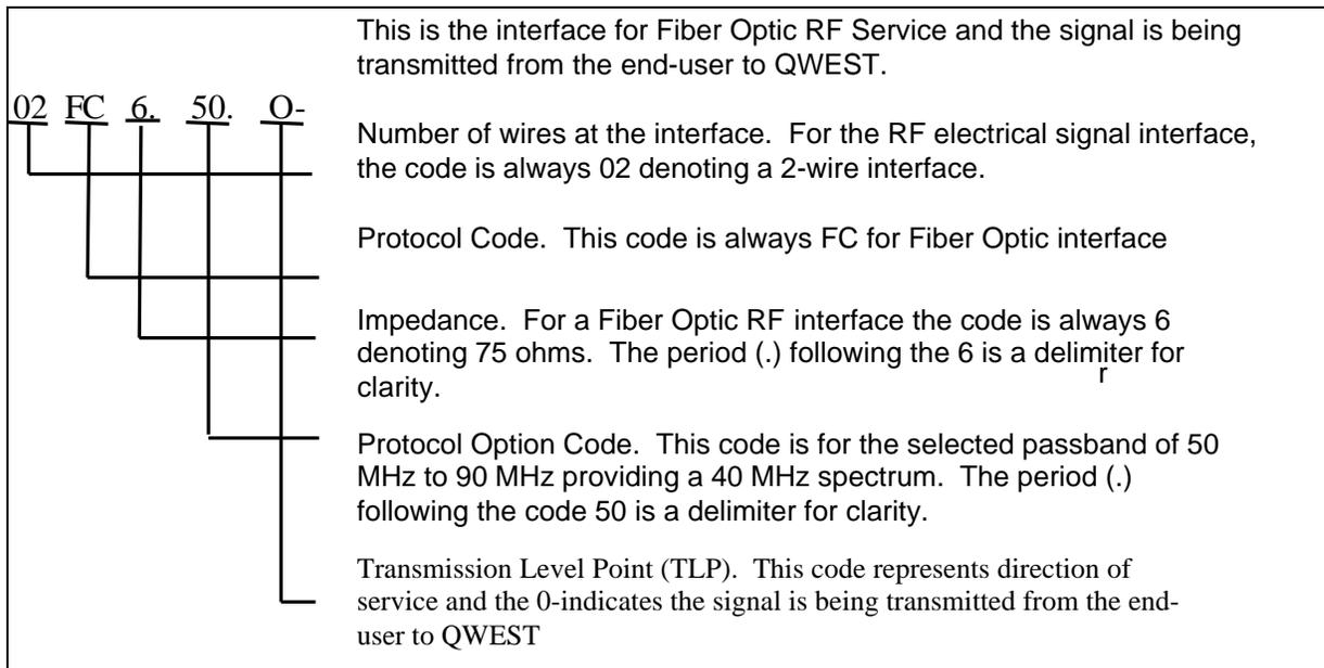
**Figure 3-1** QWEST Fiber Optic RF Service NCI Code
