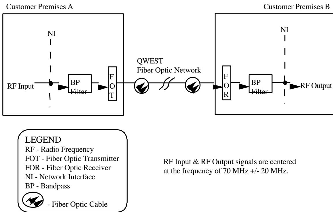
**Figure 2-1** QWEST Fiber Optic RF Service
