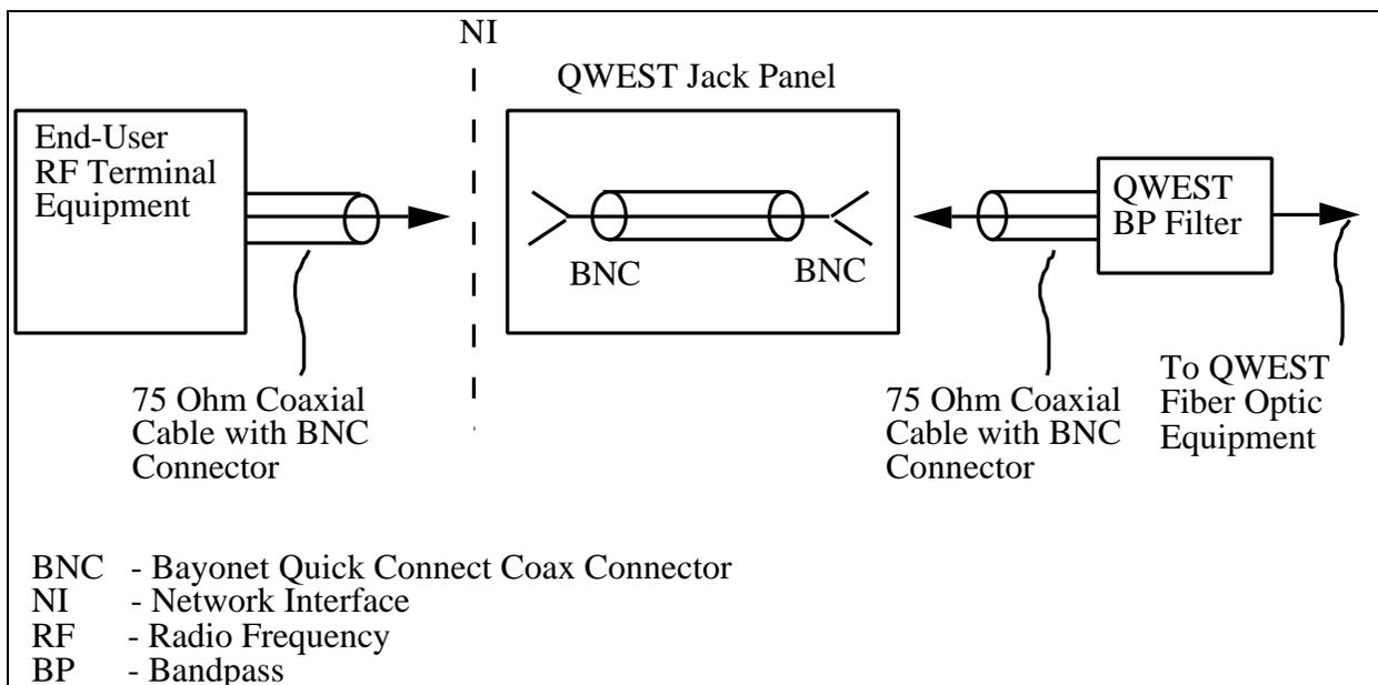
**Figure 4-1** Network Interface Connection
