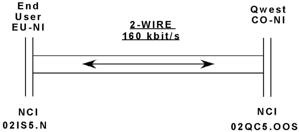
**Figure 5-3:** Typical Unbundled xDSL-I Channel
