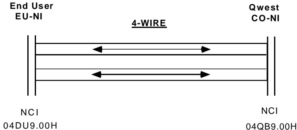
**Figure 6-2** Typical Unbundled HDSL Loop
