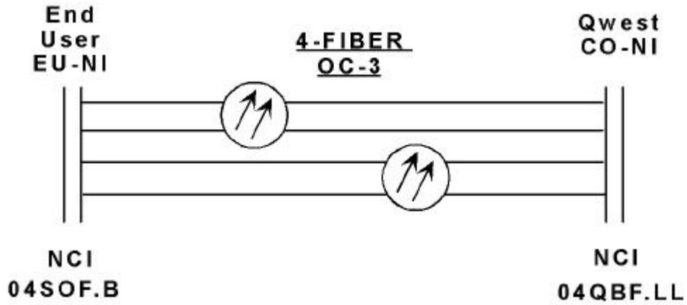
**Figure 5-6:** Typical SONET Unbundled Channel.
