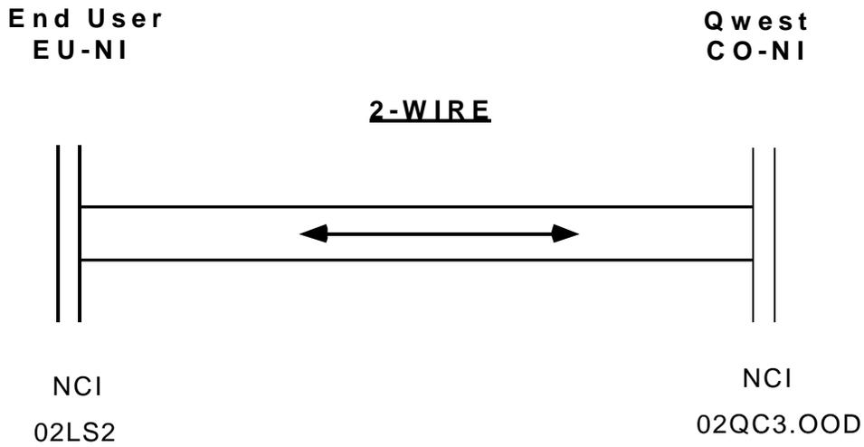
**Figure 4-1:** Typical Unbundled Voiceband Channel 2-Wire Configuration
