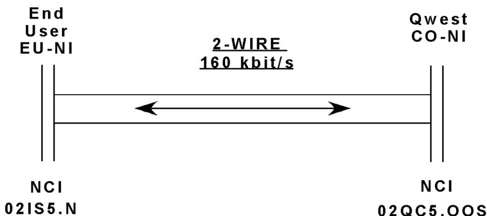
**Figure 5-2:** Typical Unbundled DSL Channel
