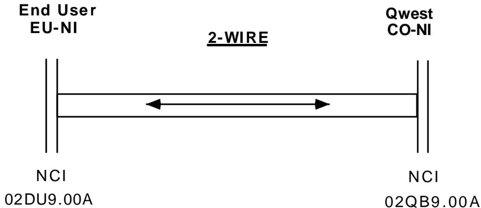
**Figure 6-3** Typical ADSL Unbundled Loop.
