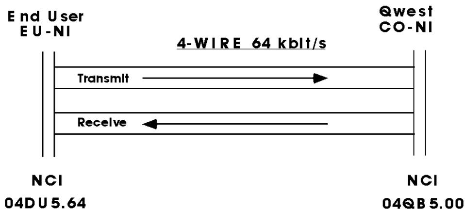
Figure 5-1: Typical Unbundled DDS Channel
