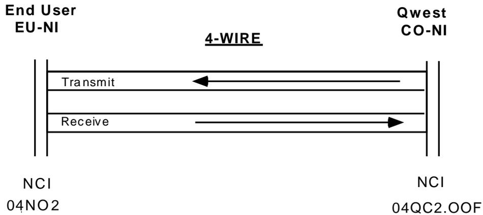
**Figure 4-2:** Typical Unbundled Voiceband Channel, 4-Wire Configuration
