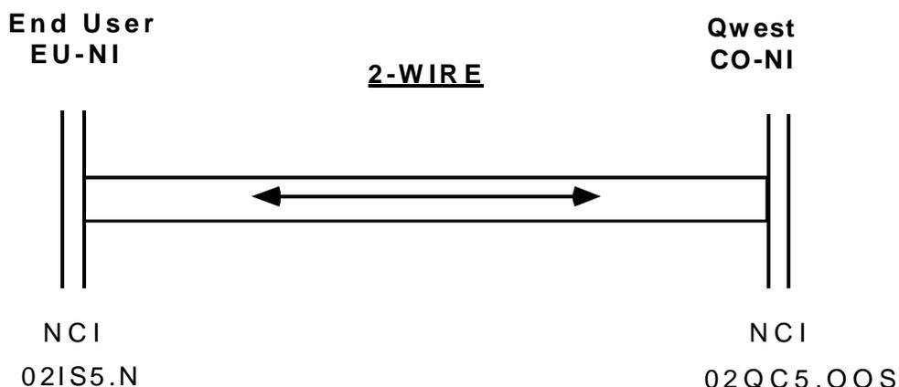
**Figure 6-1** Typical Unbundled Digital Subscriber Line (DSL) Loop
