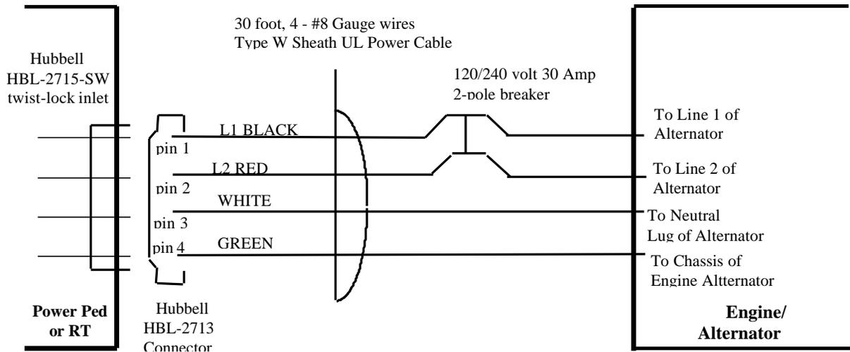
**Figure 6-1** 30-Ampere Cable Hardwired to Single-Phase Engine-Alternator
