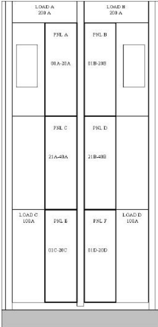
Figure 8-9 Typical Layout of 4 Load 400 Ampere BDFB
