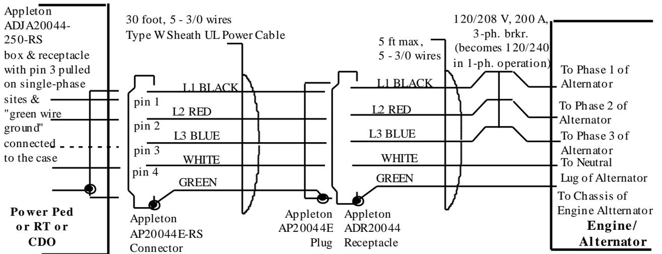
**Figure 6-10** 200-Ampere Cable To Three-Phase or Single/Three-Phase Engine-Alternator Receptacle
