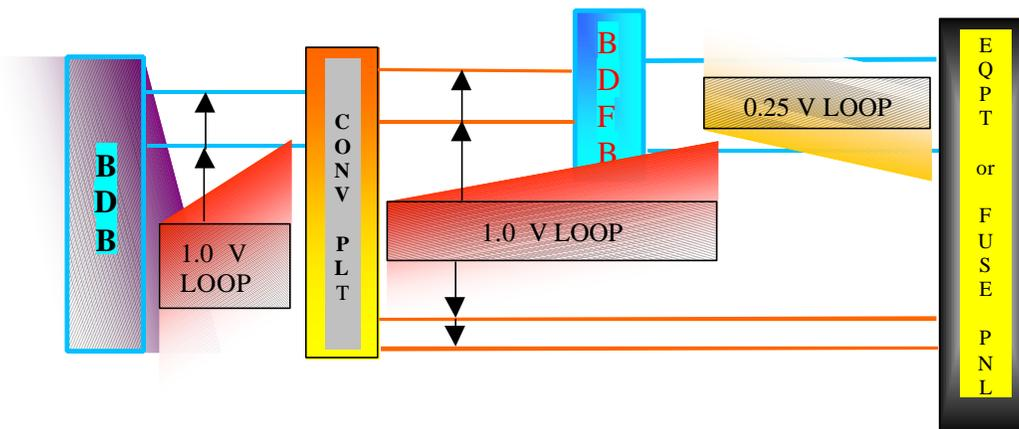
Figure 8-4 Equipment Distribution Voltage Drops for Converter Plants
