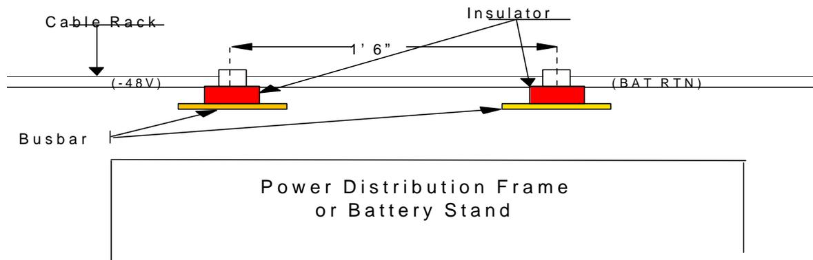
Figure 8-5 Typical Mounting of Bus Bar above PDFs and Battery Stands
