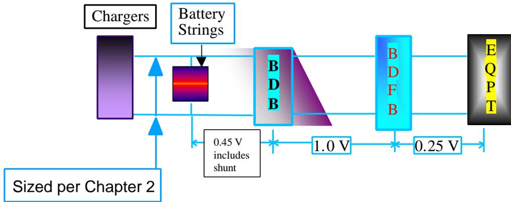
Figure 8-2 Equipment Distribution Voltage Drops Loop
