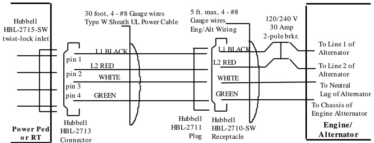
**Figure 6-2** 30-Ampere Cable to Single-Phase Engine-Alternator Receptacle
