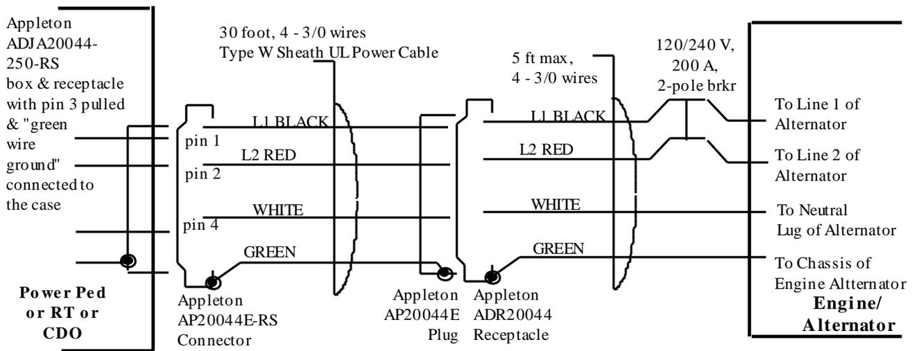
Figure 6-8 200-Ampere Cable to Single-Phase Engine-Alternator Receptacle
