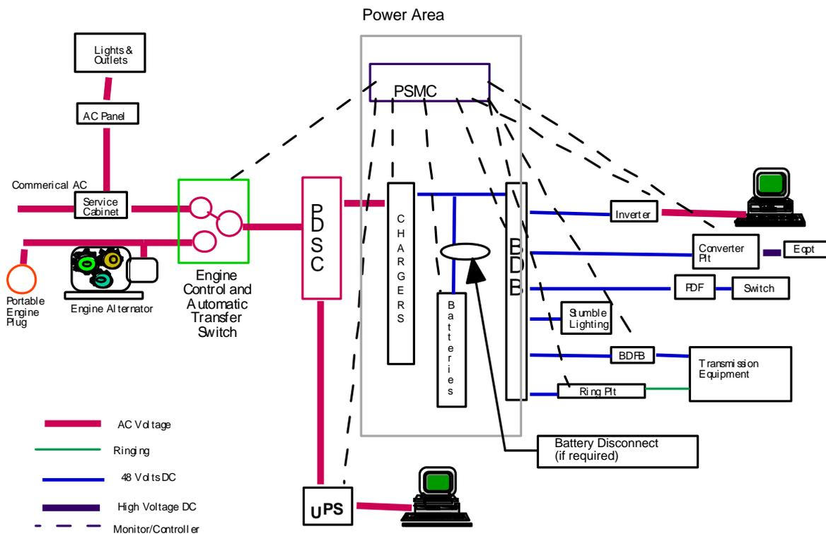
**Figure 2-1** A Powering Scheme for a Central Office
