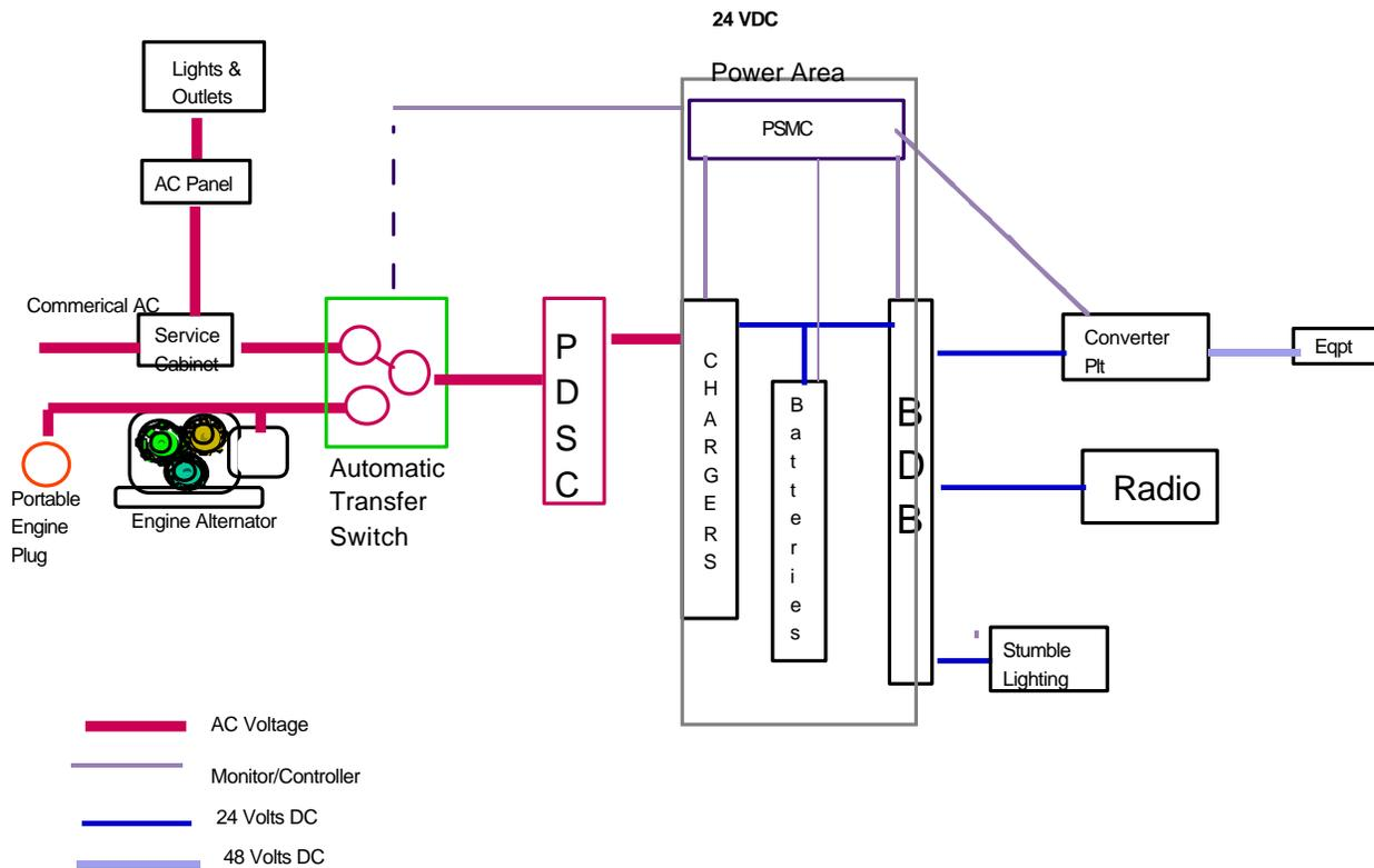
Figure 2-3 Typical Radio Site Power Scheme
