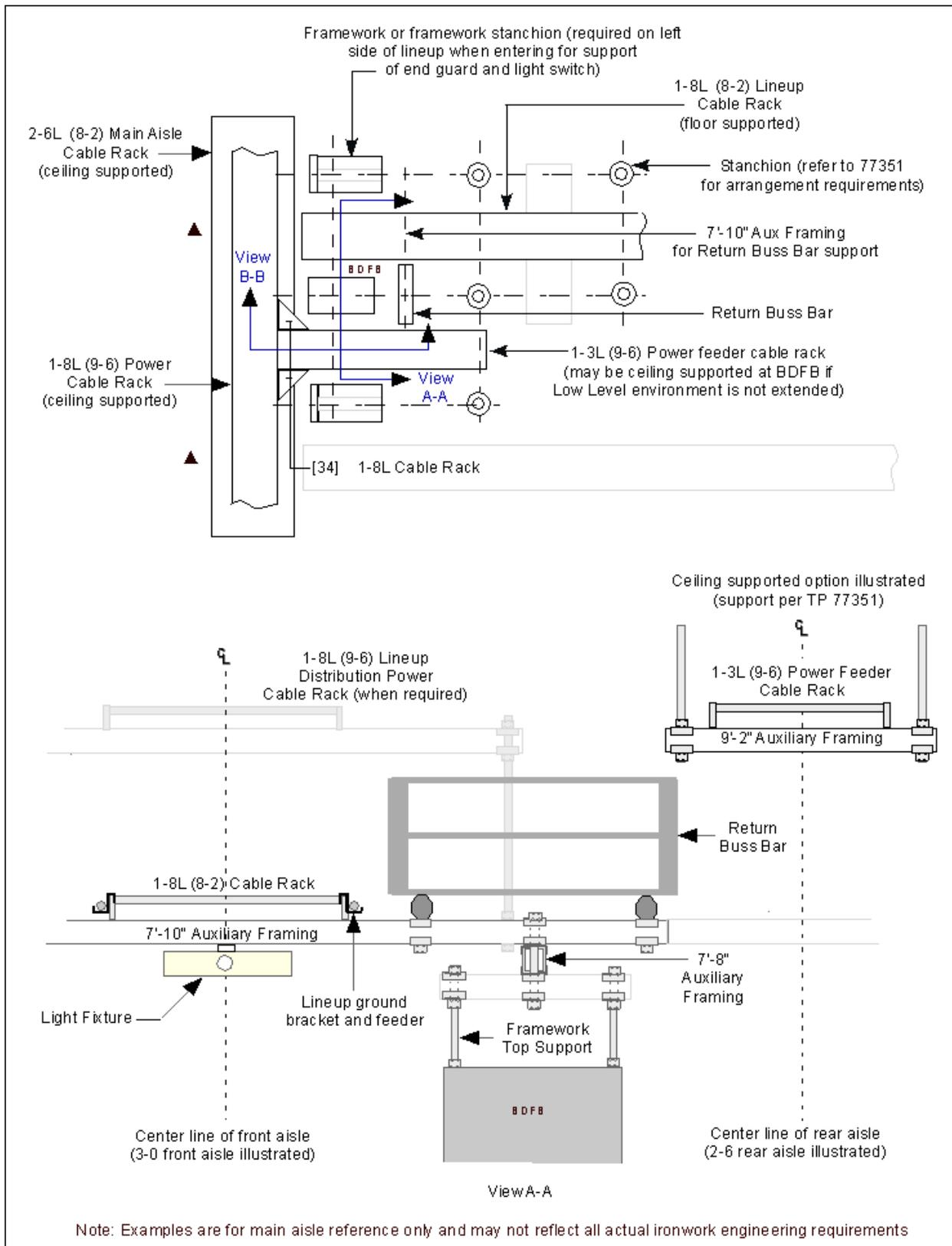
Figure 8-10 Typical Return Bus Bar Mounting for a 7' BDFB (View A-A)
