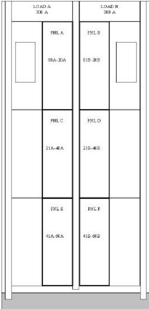
Figure 8-8 Typical Layout of 2 Load 600 Ampere BDFB
