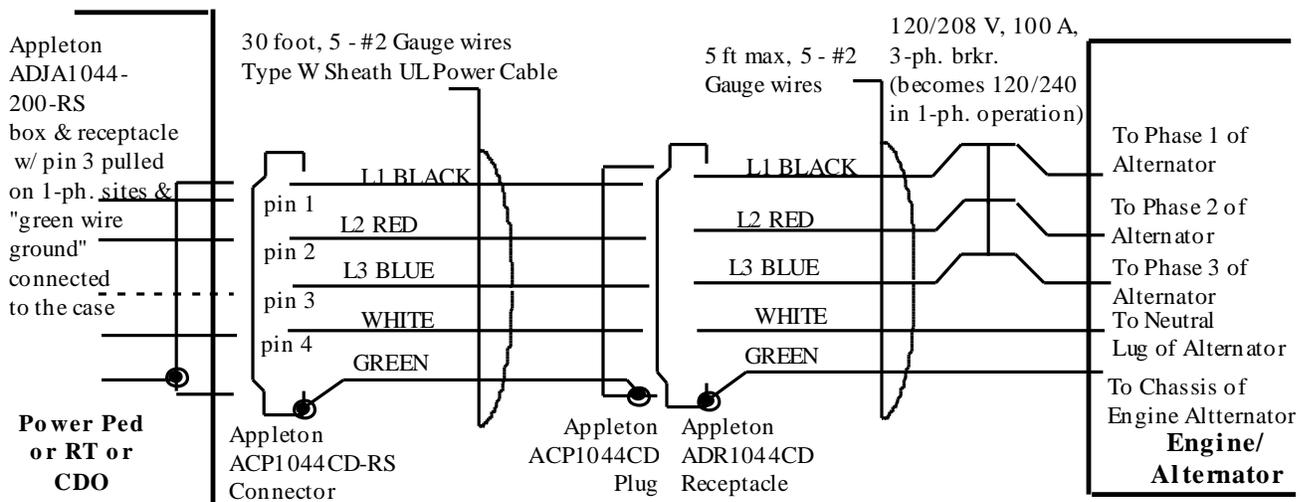
**Figure 6-6** 100-Ampere Cable To Three-Phase or Single/Three-Phase Engine-Alternator Receptacle
