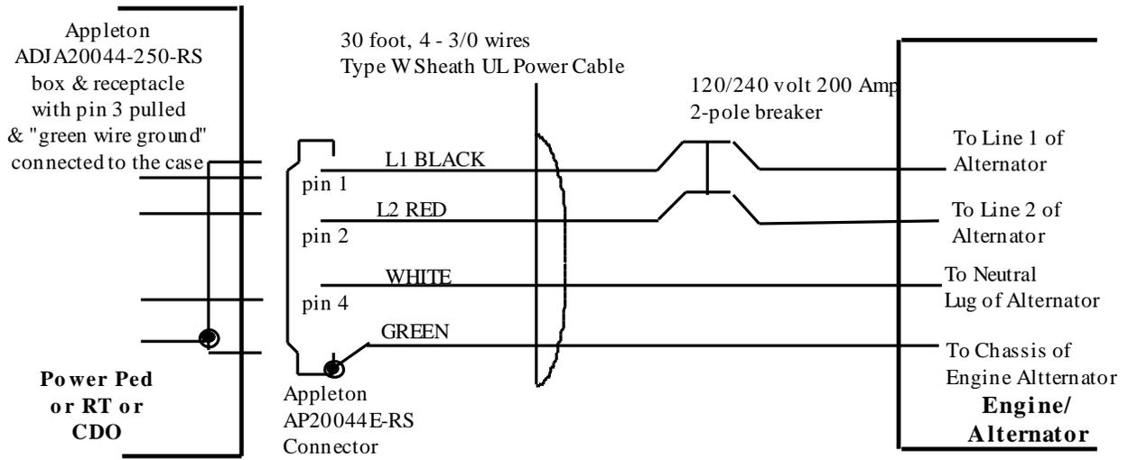
Figure 6-7 200-Ampere Cable Hardwired to Single-Phase Engine-Alternator
