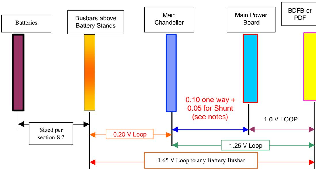
Figure 8-3 Voltage Drops from Battery Strings to BDBs
