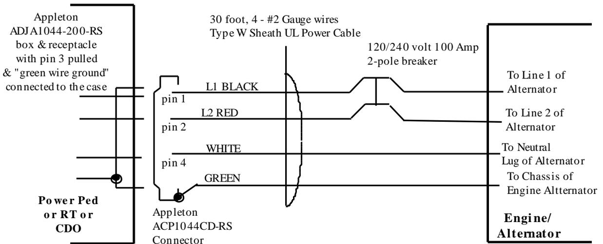
**Figure 6-3** 100-Ampere Cable Hardwired to Single-Phase Engine-Alternator
