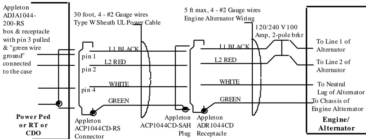
**Figure 6-4** 100-Ampere Cable to Single-Phase Engine-Alternator Receptacle
