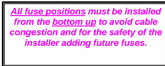
Figure 8-6 BDFB Fuse Assignment Label
