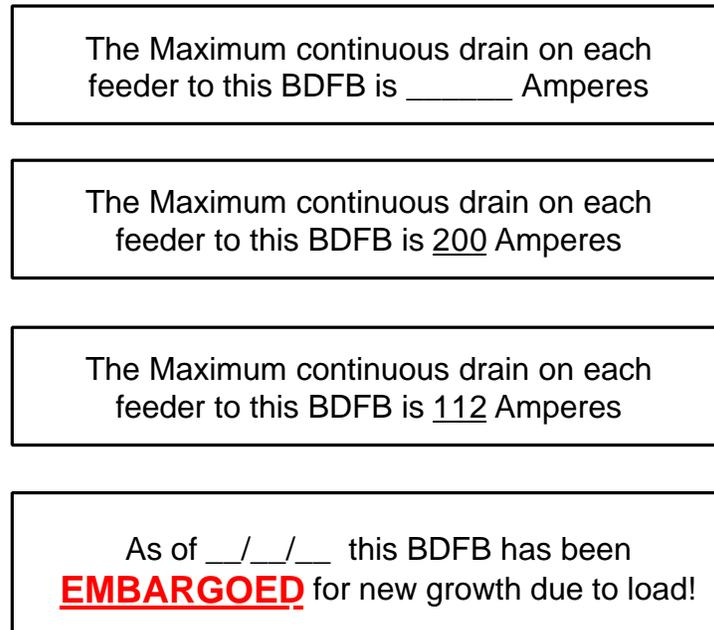
Figure 8-12 Load and Embargo Labels for BDFBs
