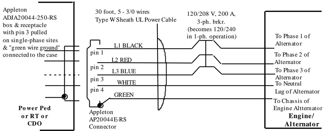
**Figure 6-9** 200-Ampere Cable Hardwired To Three-Phase or Single/Three-Phase Engine-Alternator
