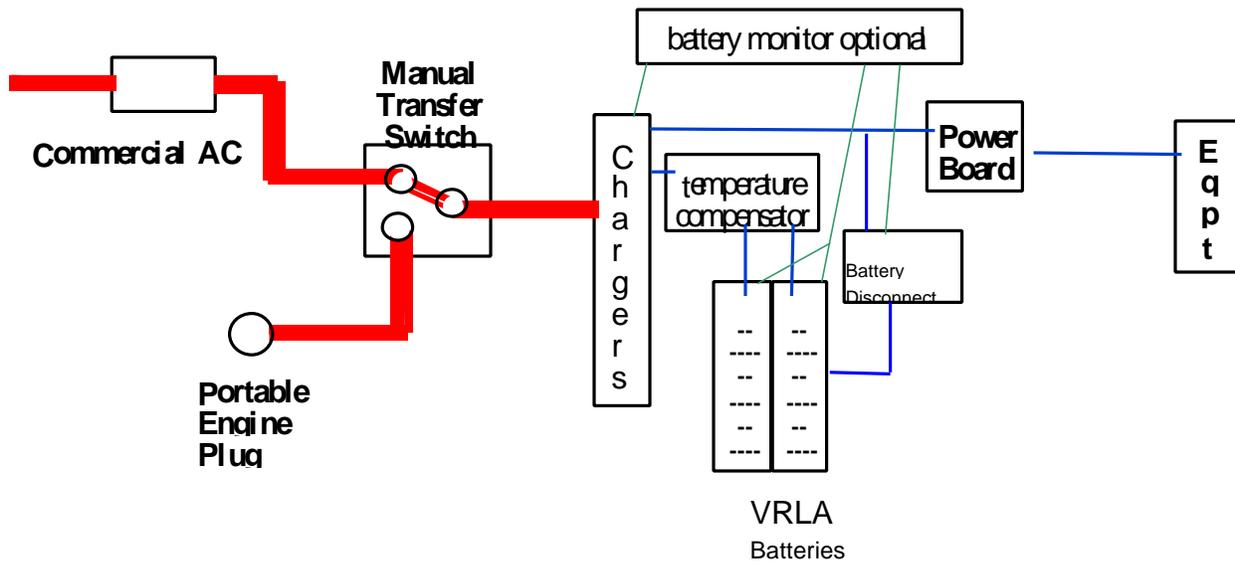
Figure 2-2 Typical Outside Plant Equipment Enclosure Power Scheme
