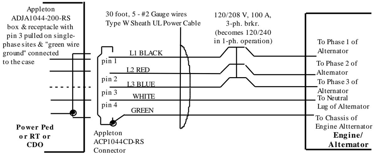
**Figure 6-5** 100-Ampere Cable Hardwired To Three-Phase or Single/Three-Phase Engine-Alternator
