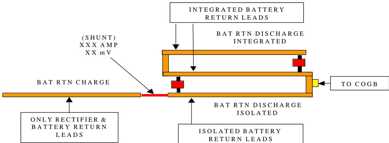
Figure 8-18 Main Return/Ground Window Bar in Power Room
