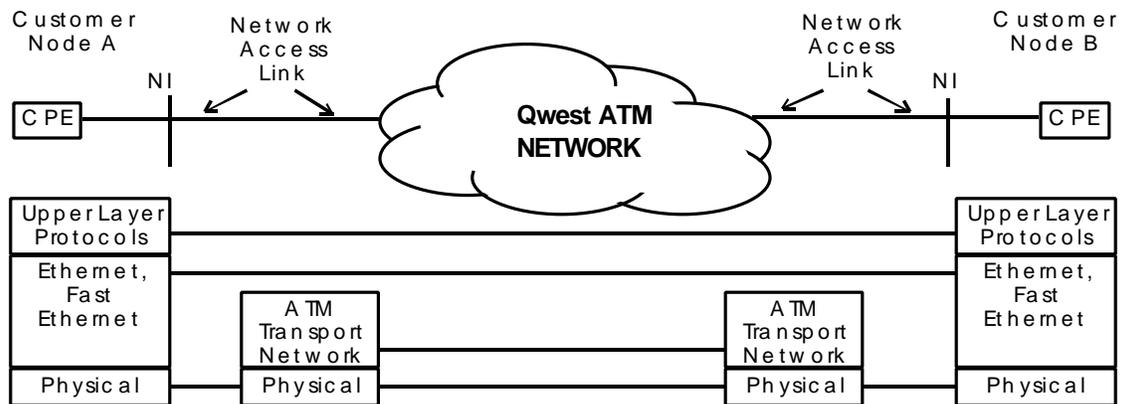
**Figure 2-2: Relationship between LSS Nodes and the QWEST ATM Network**
