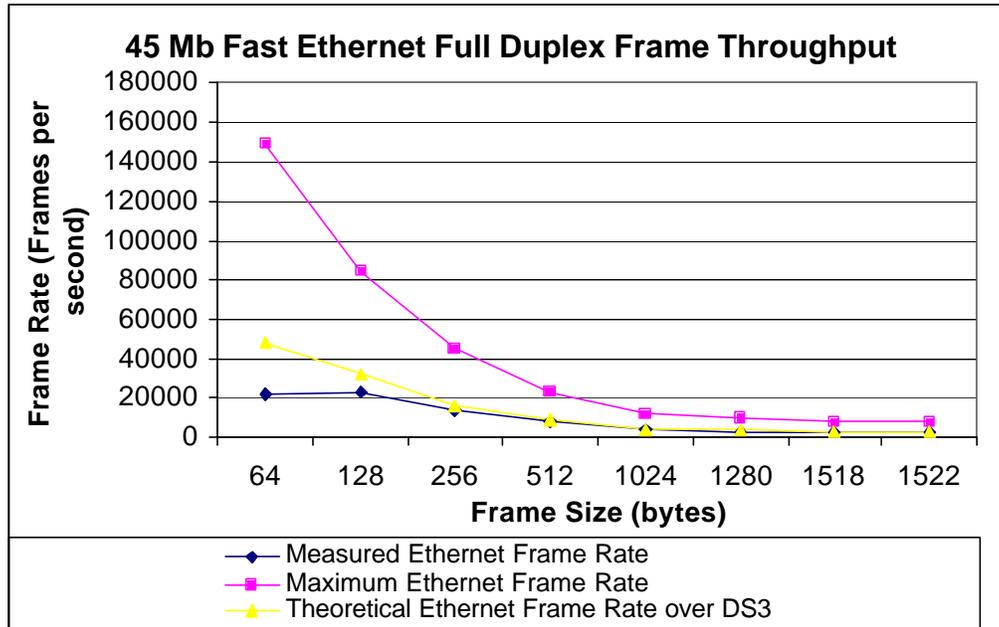
**Figure 4-5:** 45 Mb Fast Ethernet Full Duplex (PLCP) Throughput in FPS
