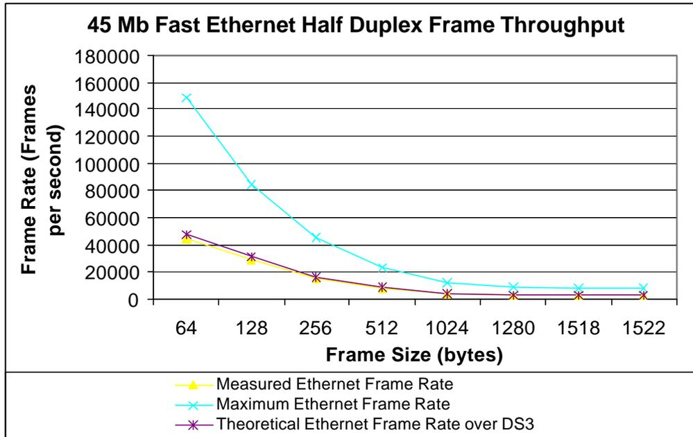
**Figure 4-3:** 45 Mb Fast Ethernet Half Duplex (PLCP) Throughput in FPS
