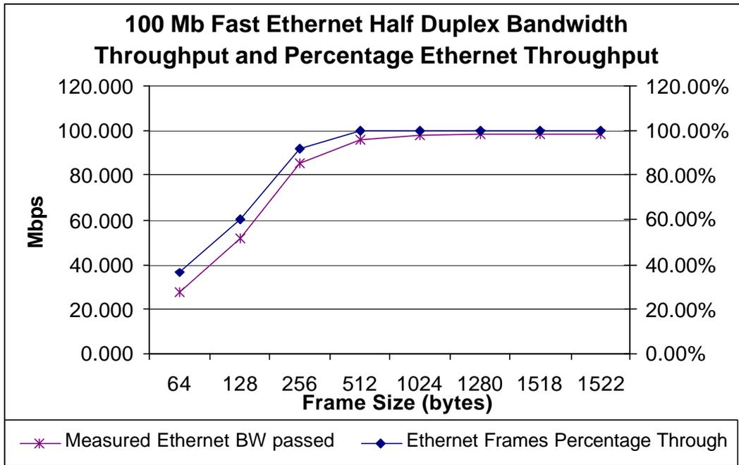
Figure 4-8: 100 Mb Fast Ethernet Half Duplex Throughput in Mbps and Percentage Throughput
