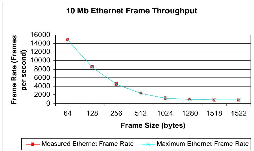
**Figure 4-1:** 10 Mb Ethernet Throughput in Frames per second (FPS)
