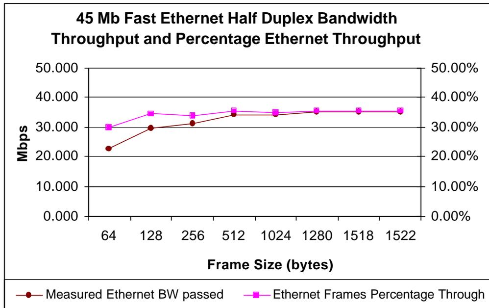
**Figure 4-4:** 45 Mb Fast Ethernet Half Duplex (PLCP) Throughput in Mbps and Percentage Throughput
