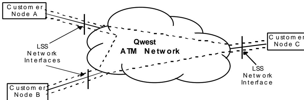
**Figure 2-3:** Example of LSS Node Networking Using Multiple Virtual Circuits.
