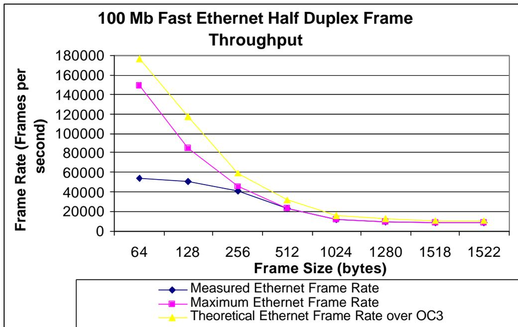
Figure 4-7: 100 Mb Fast Ethernet Half Duplex Throughput in FPS
