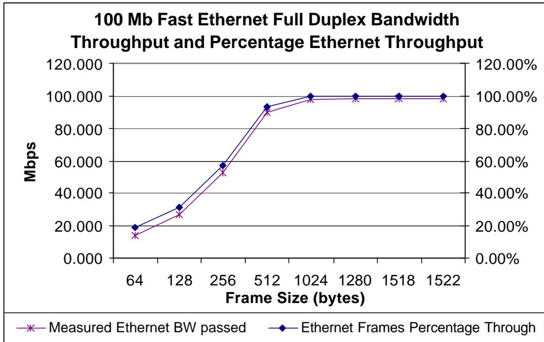
**Figure 4-10:** 100 Mb Fast Ethernet Full Duplex Throughput in Mbps and Percentage Throughput
