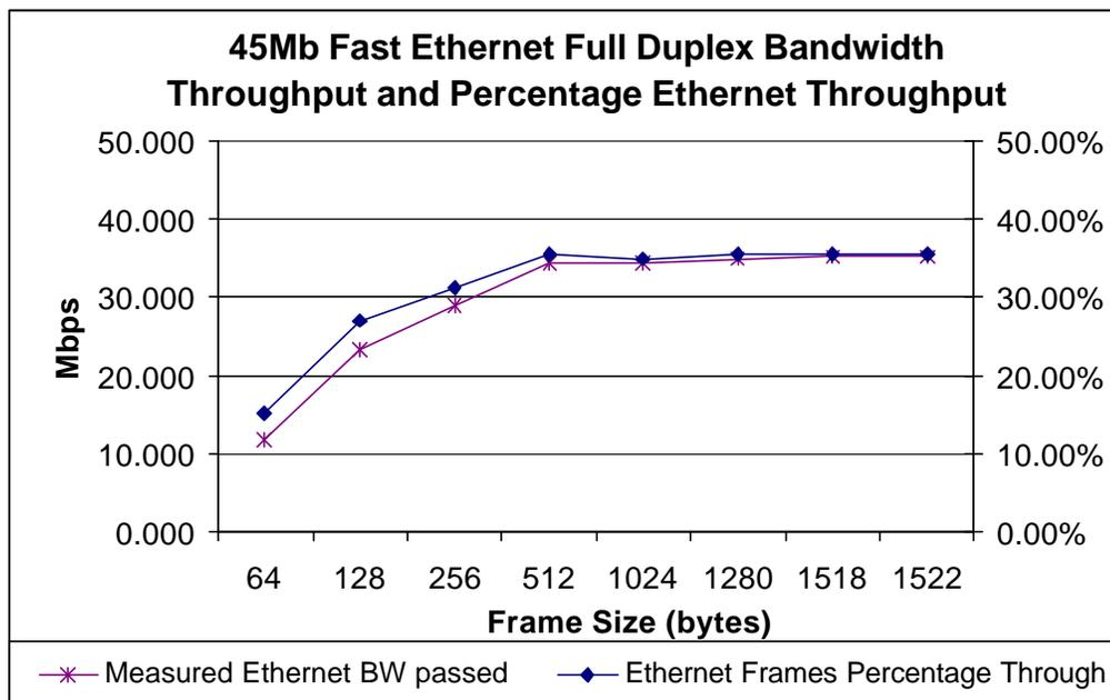
**Figure 4-6:** 45 Mb Fast Ethernet Full Duplex (PLCP) Throughput in Mbps and Percentage Throughput
