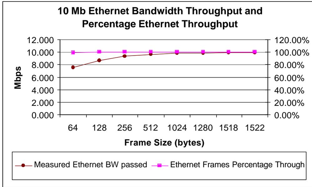
**Figure 4-2: 10 Mb Ethernet Throughput in Mbps and Percentage Throughput**
