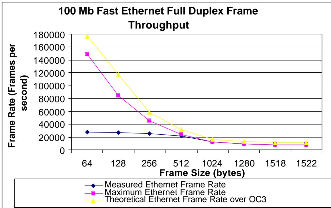
Figure 4-9: 100 Mb Fast Ethernet Full Duplex Throughput in FPS
