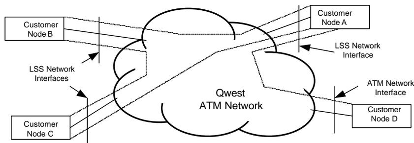
**Figure 2-4:** Example of LSS to ATM Networking Using a Virtual Circuit.
