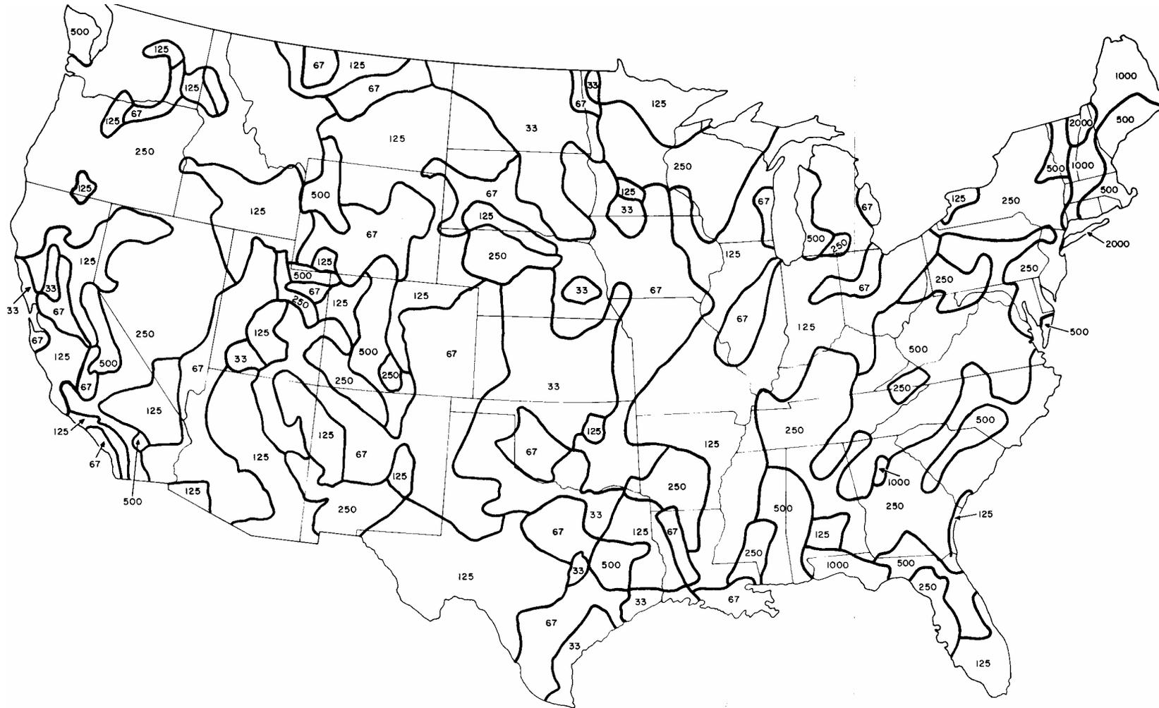
Figure 1 –Estimated Average Earth Resistivity in the U. S. (Meter-Ohms)
