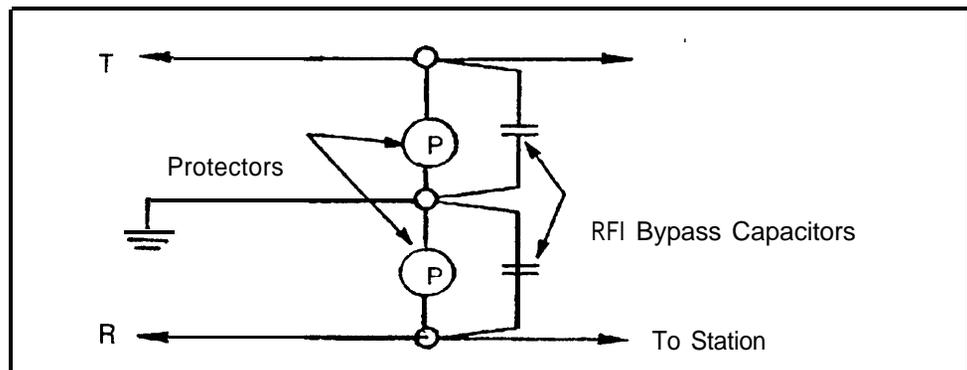
**NOTE:** Sometimes capacitors might be effective in suppressing Amateur Band and CB signals (up to 27 MHz).
