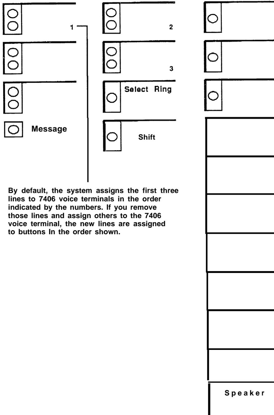
By default, the system assigns the first three lines to 7406 voice terminals in the order indicated by the numbers. If you remove those lines and assign others to the 7406 voice terminal, the new lines are assigned to buttons in the order shown.
