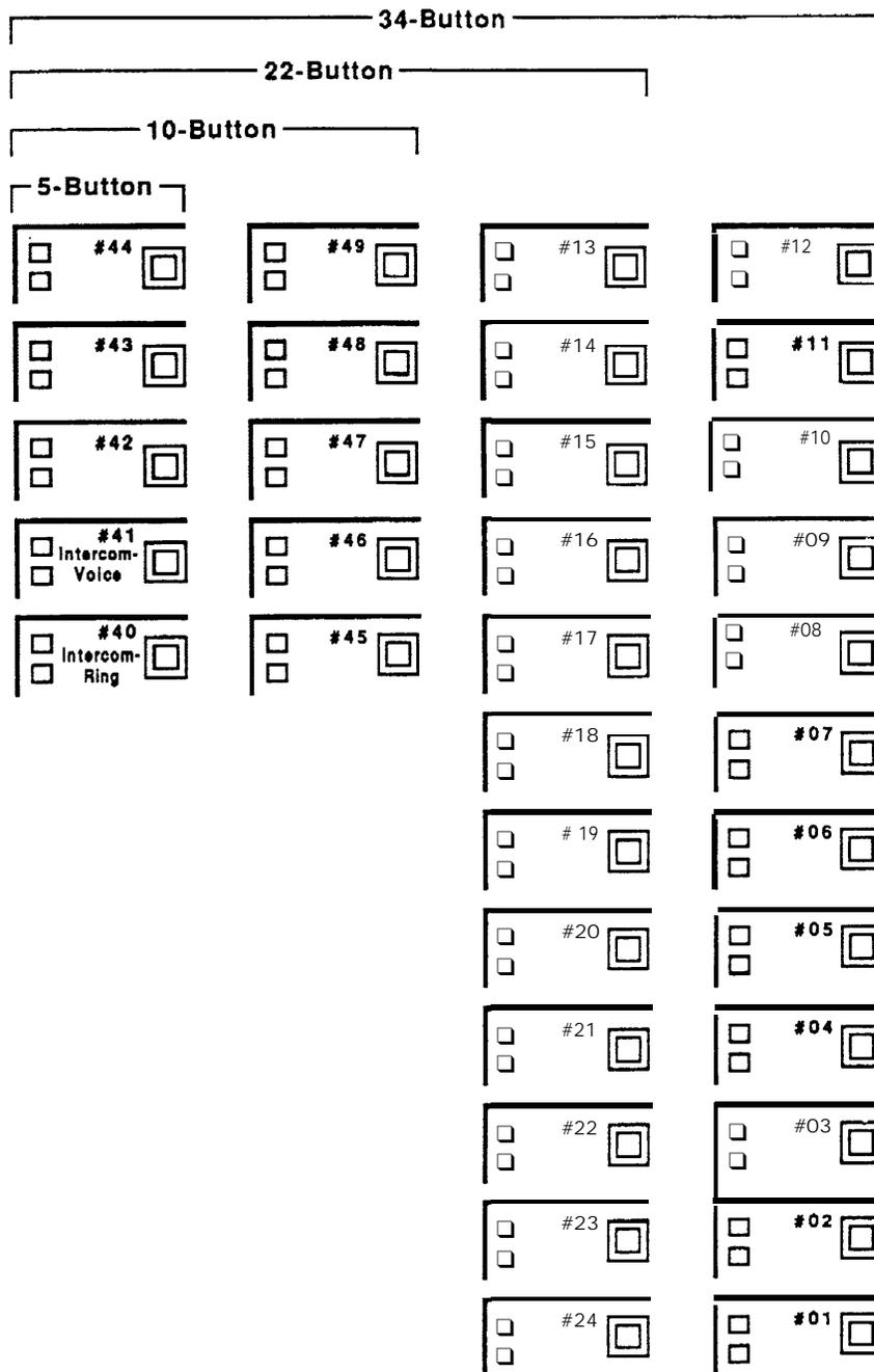
FIGURE 2-2 Button location codes for digital 7406 voice terminals.
