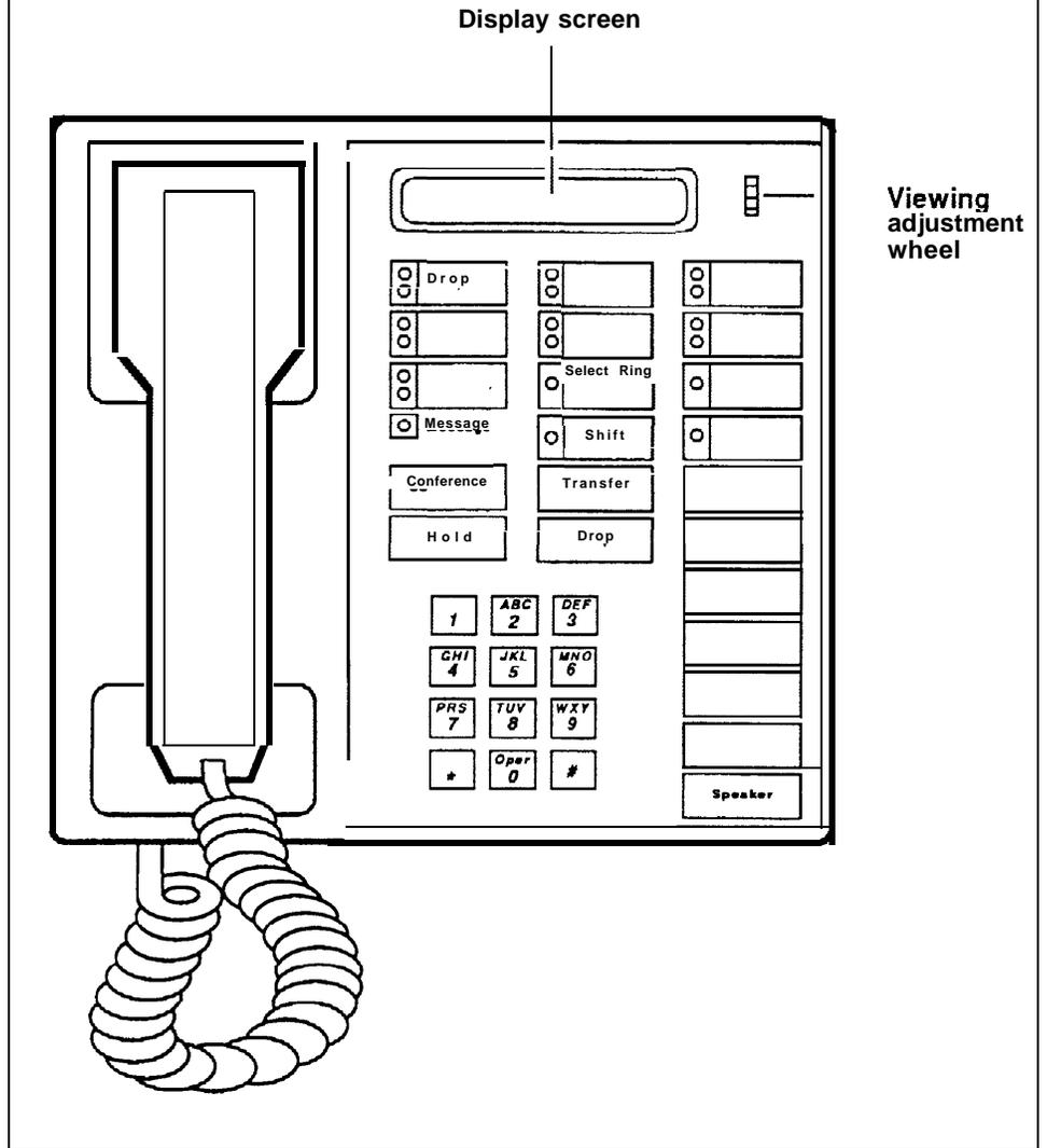
FIGURE 2-5 The MERLIN II System Display Console
