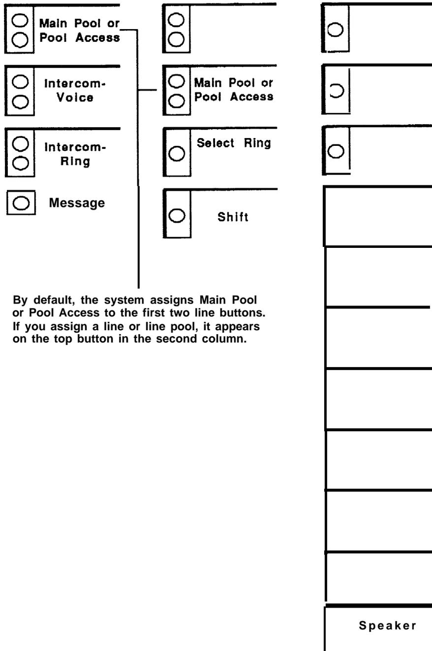
By default, the system assigns Main Pool or Pool Access to the first two line buttons. If you assign a line or line pool, it appears on the top button in the second column.
