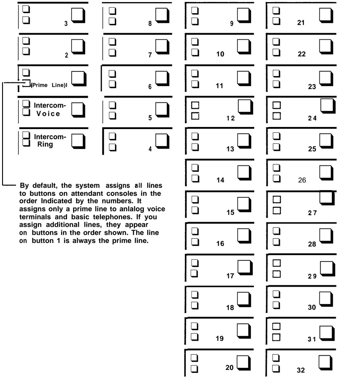
**FIGURE 2-8** The order in which secondary lines preassigned to buttons on digital voice terminals.
