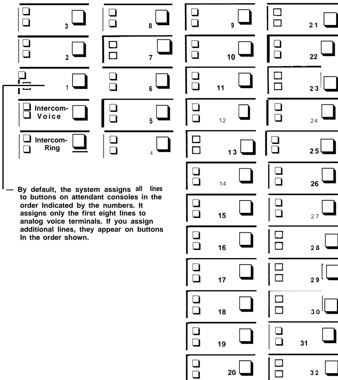
**FIGURE 2-12** The order in which lines are assigned to buttons on digital voice terminals in a square configuration.
