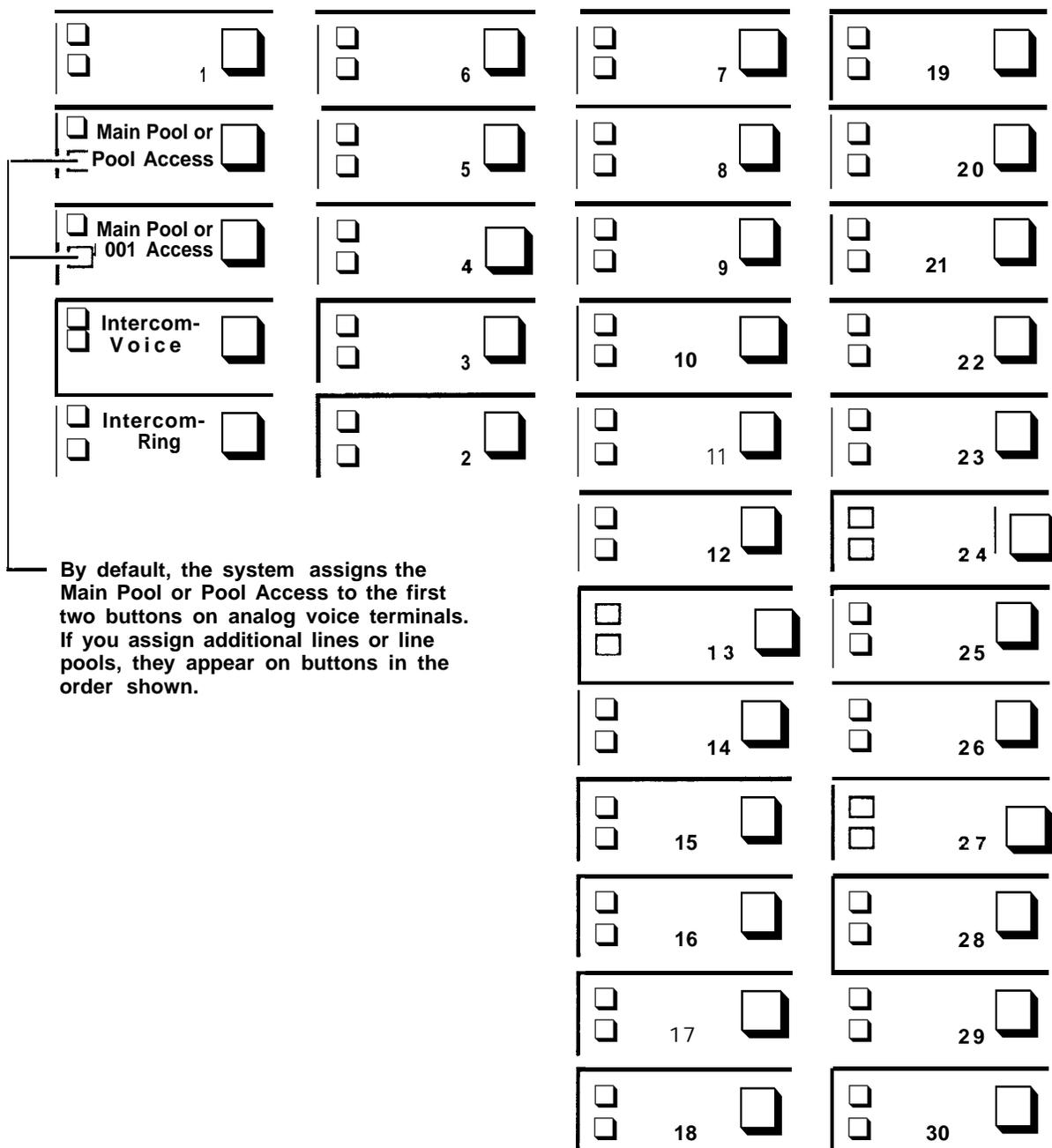
**FIGURE 2-10** The order in which lines and line pools are assigned to digital voice terminals.
