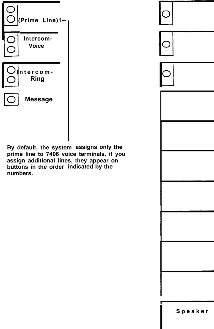
By default, the system assigns only the prime line to 7406 voice terminals. if you assign additional lines, they appear on buttons in the order indicated by the numbers.
