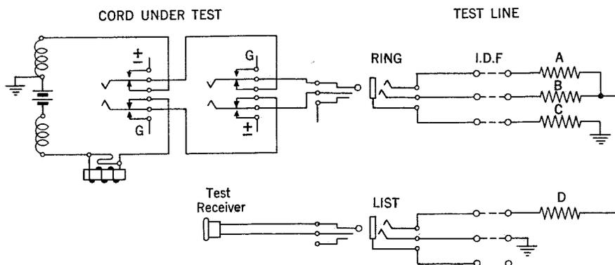
Fig. 1 - Test of Ringing Key Contacts.
