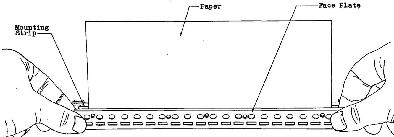
Fig. 3 - Method of Assembling Face Plate on Mounting Strip
