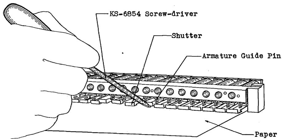
Fig. 2 - Method of Checking Location of Shutters
