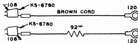
The code of the cord includes two KS6780 connecting clips with two No. 108 cord tips (rubber insulators), and two No. 120 cord tips.
