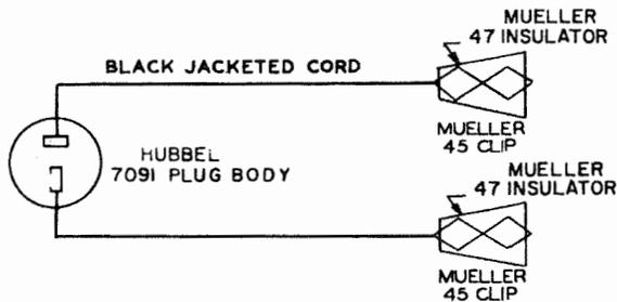
The code of the cord includes the No. 7091 Hubbell body, two No. 45 Mueller clips, and two No. 47 Mueller insulators.
