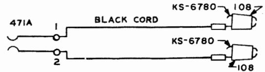
The individual code of the cord includes two KS6780 connecting clips with two No. 108 cord tips (rubber insulators).
