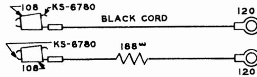
The code of the cord includes two KS6780 connecting clips with two No. 108 cord tips (rubber insulators), and two No. 120 cord tips.
