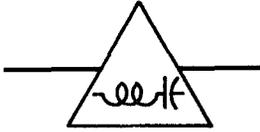
(4) L-C circuit with infinite susceptance at resonance
