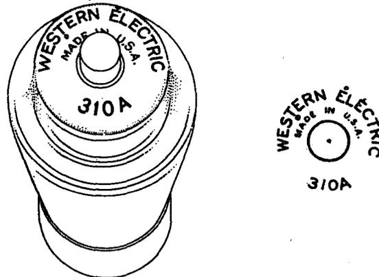
Fig. 4 - Typical Example of Bulb Marking for Tubes Having External Grid Caps
