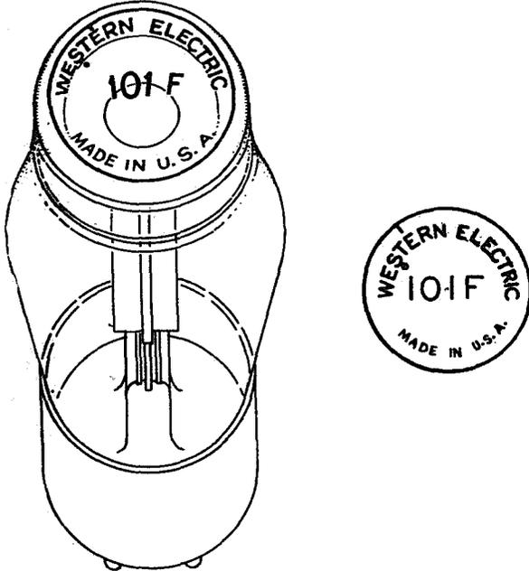
Fig. 2 - Typical Example of Bulb Marking
