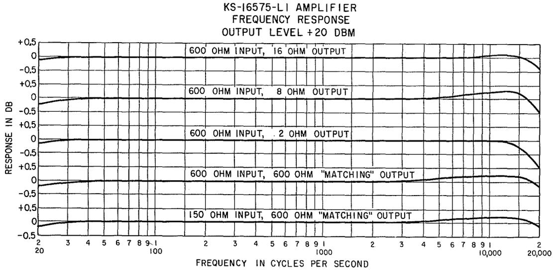
**Fig. 3A – Amplifier Frequency Response**
