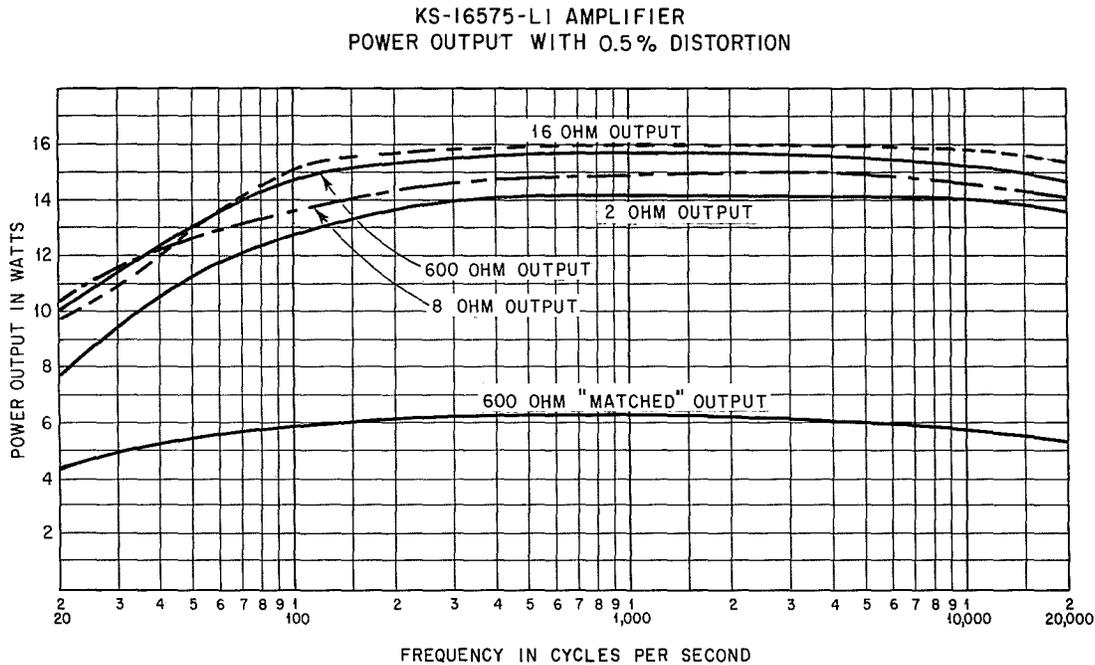
**Fig. 3B – Amplifier Distortion Characteristics**
