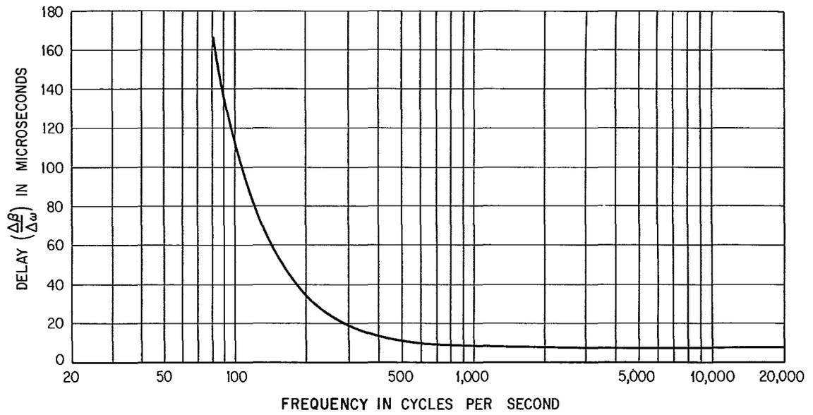
Fig. 3C – Envelope Delay Distortion
