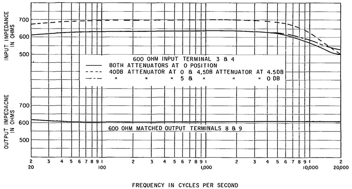
Fig. 3D – Internal Amplifier Impedances
