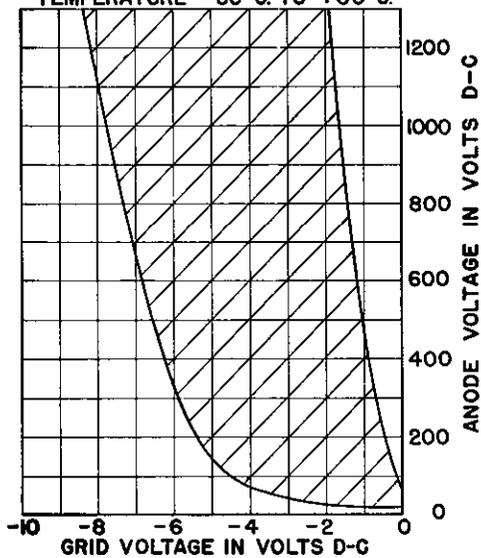
TYPICAL GRID CURRENT CHARACTERISTICS DURING ANODE CONDUCTION
