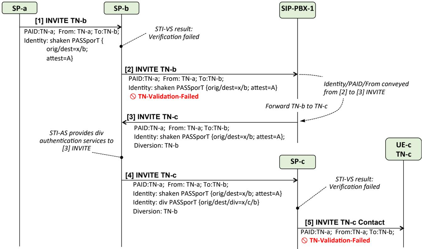
Figure A.6 – Case-1c – [1] INVITE contains invalid Identity header
