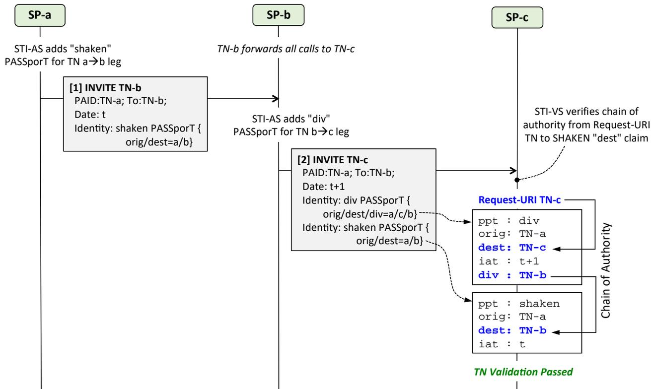
Figure 4.1 – Using "div" PASSporT to authenticate the forwarding leg of call
