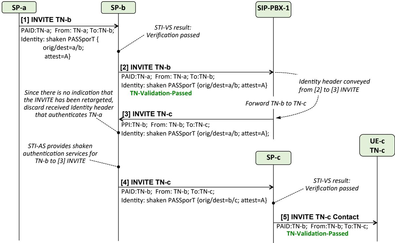
**Figure A.7 – Case-2a – [1] INVITE contains valid Identity header**
