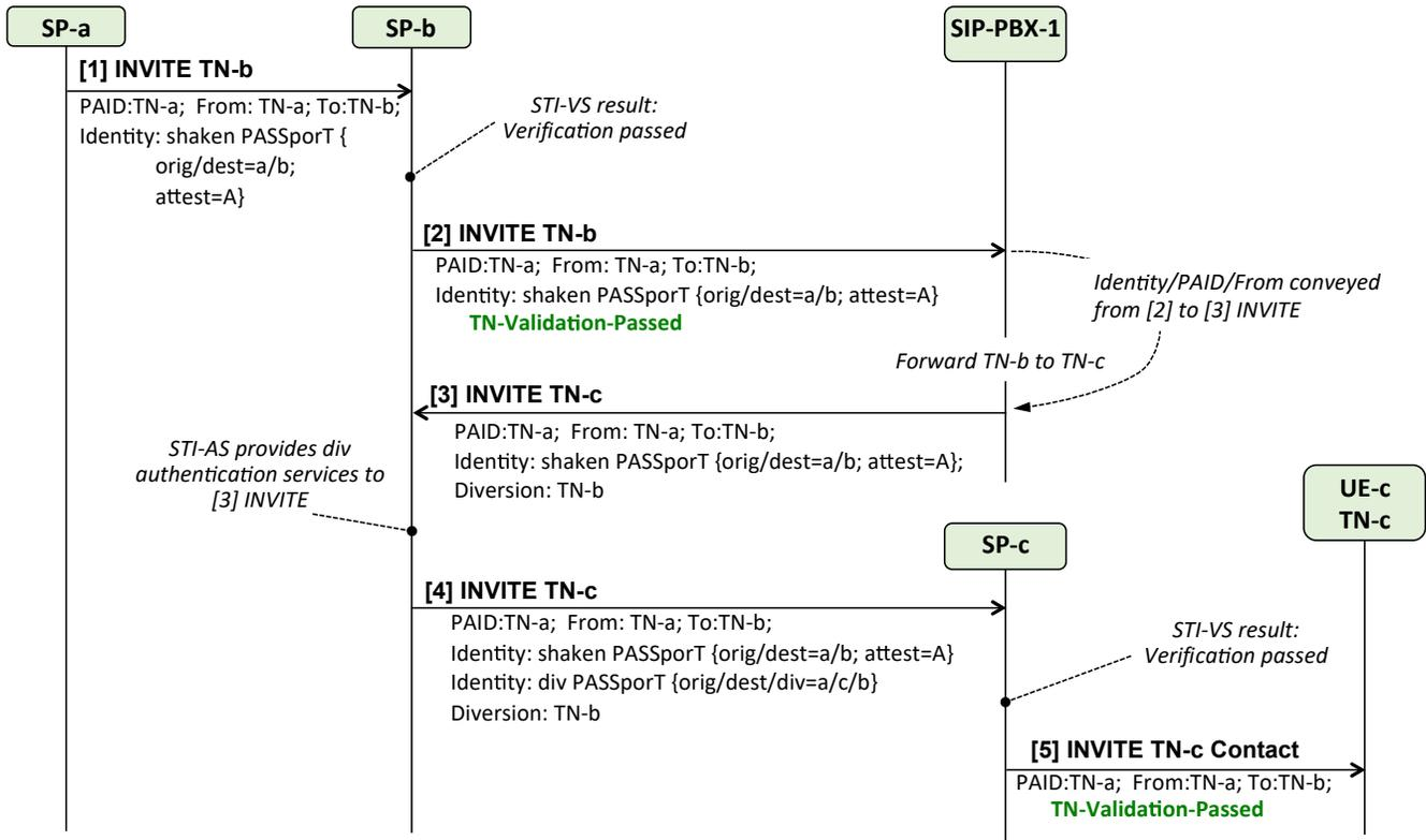
Figure A.4 – Case-1a– [1] INVITE contains valid Identity header
