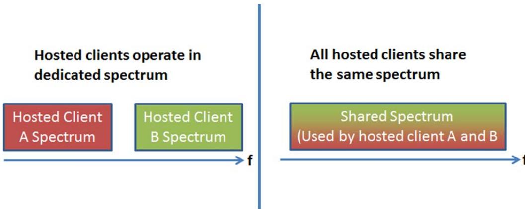
Figure 6.2 – Example Approaches to Spectrum Management in MOCN
