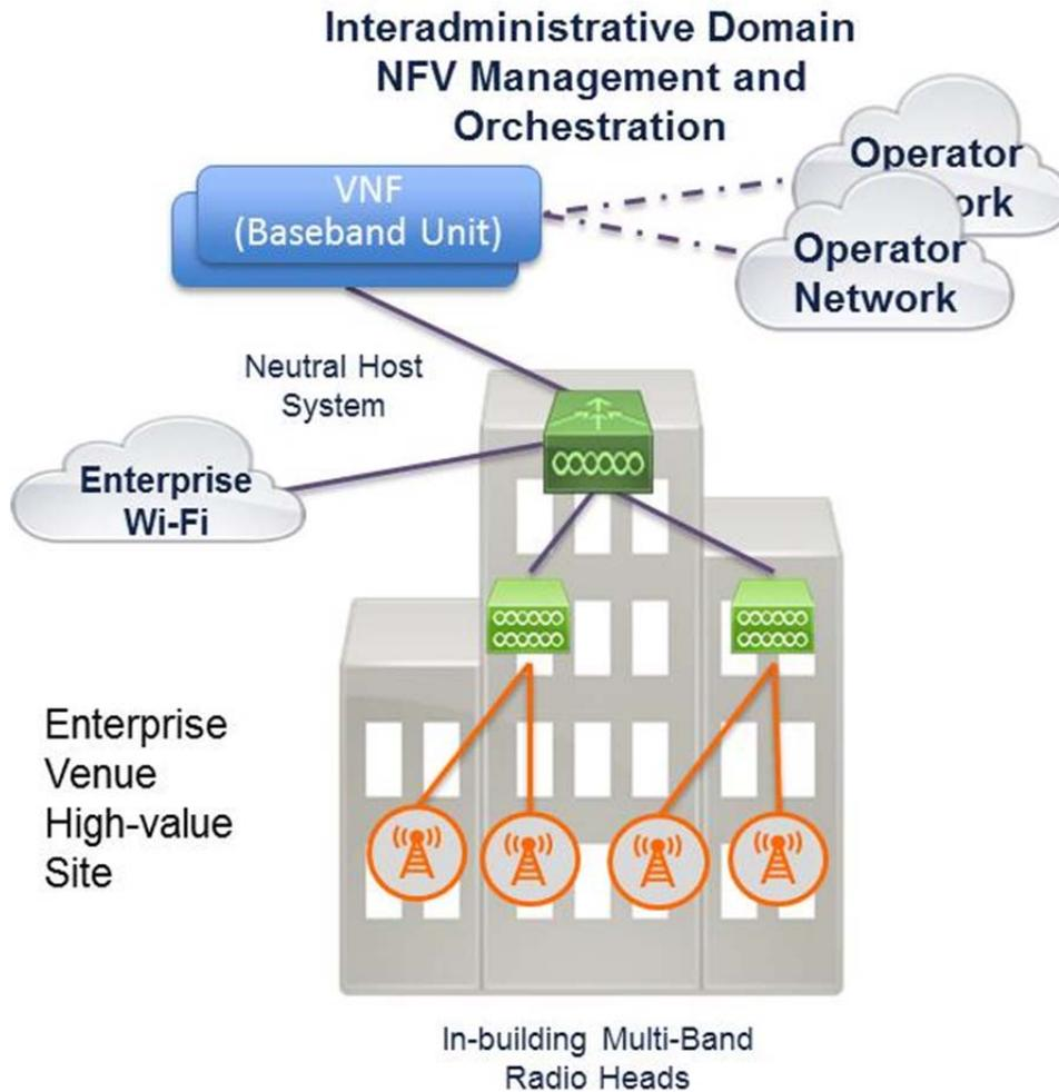
Figure 6.4 – Cloud RAN Based Neutral Host Solution
