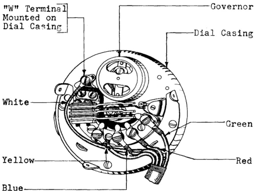
Fig. 4 - Method of Cording Dials Having a Separate "W" Terminal Mounted Directly on the Dial Casing, Using D5P or 765 Cords
