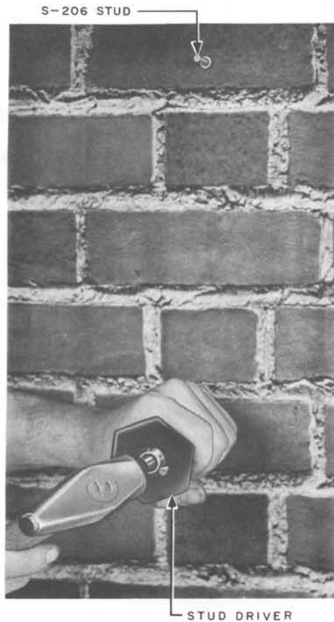
Fig. 3 — Mounting Studs
