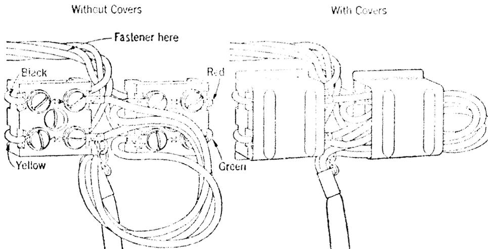
For five-conductor cords use one three-post and one two-post connecting block.
