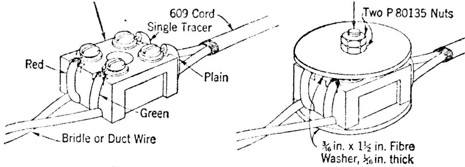
Note: Do not fasten connecting block to outlet box.
