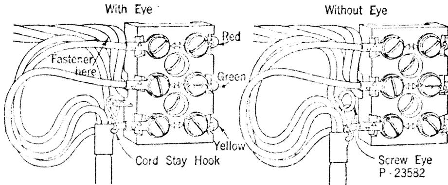
Where a connecting block without eye is used, place a screw eye for fastening cord, as shown. After fastening cord to block or screw eye, pinch opening on cord stay hook together with pliers.
