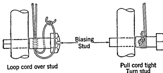
**Fig. 11—Attaching Biasing Springs on Ringers**
