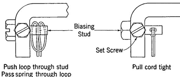
**Fig. 12—Attaching Biasing Springs on 392-Type Loud Ringing Bells**
