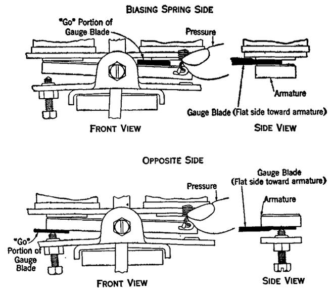
Fig. 7—Method of Checking Airgaps on 392-Type Subscriber Sets (Loud Ringing Bells)
