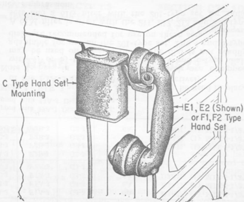
**Fig. 2—Typical 201-Type Hand Telephone Set**
