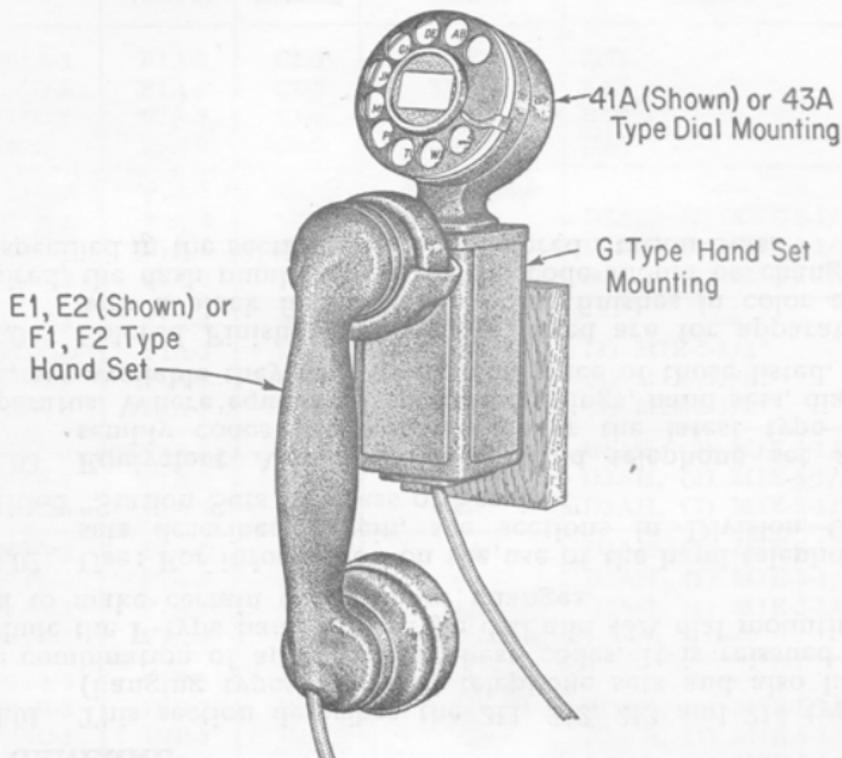
Fig. 1—Typical 211, 212, 213 and 214 Hand Telephone Sets
