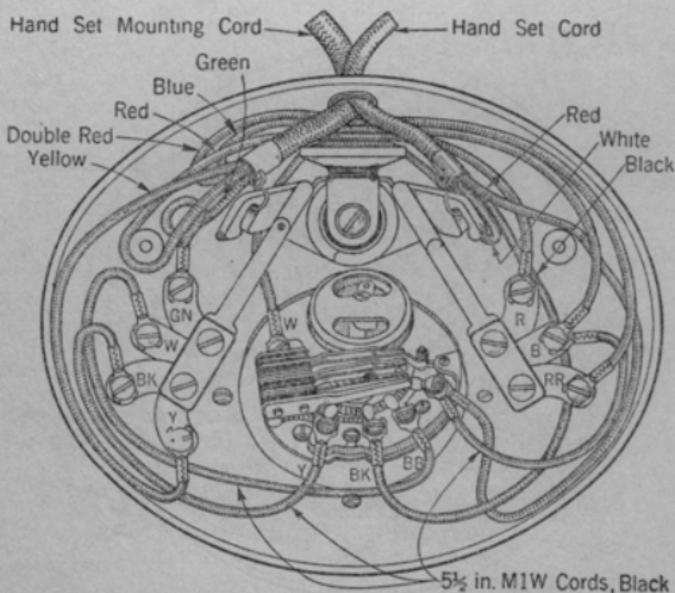
Fig. 1—D2 Type Hand Set Mounting.
