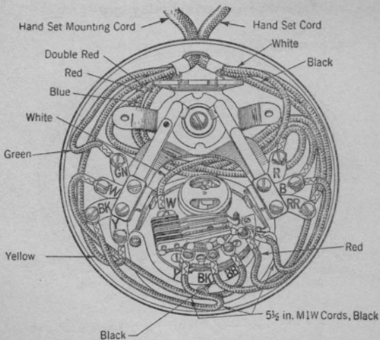
**Fig. 2—B2 Type Hand Set Mounting.**
