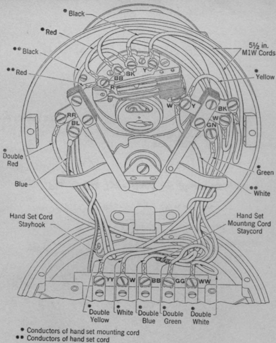
**Fig. 3—E7 Type Hand Set Mounting.**
