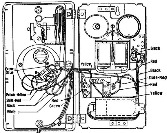
Fig. 5 — 356C Telephone Set with 6 Type Dial
