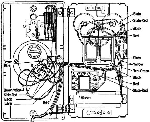
Fig. 3 — 354C Telephone Set with 6 Type Dial
