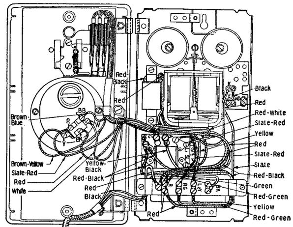
Fig. 7 — 357C Telephone Set with 6 Type Dial
