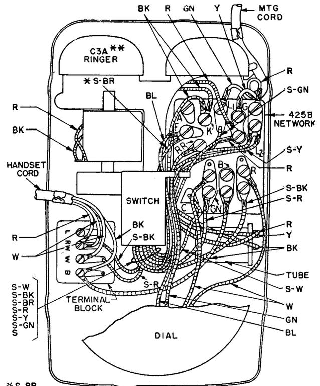
Fig. 18—501C (Manual) and 501D (Dial) Telephone Sets Converted from 501J/K Telephone Sets—Cording
