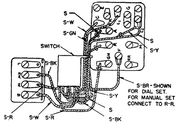
Fig. 5B—500J (Manual) and 500K (Dial) Telephone Sets—Switch Detail
