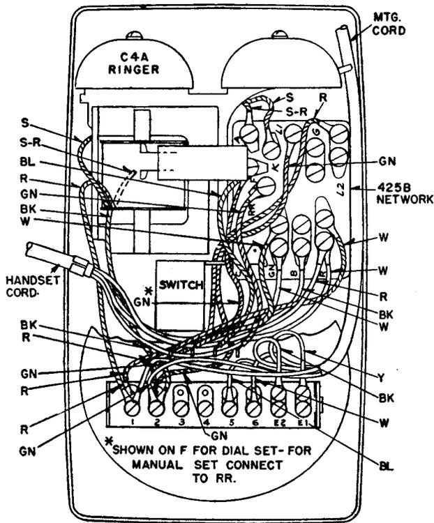
Fig. 14A—502A (Manual) and 502B (Dial) Telephone Sets—Cording
