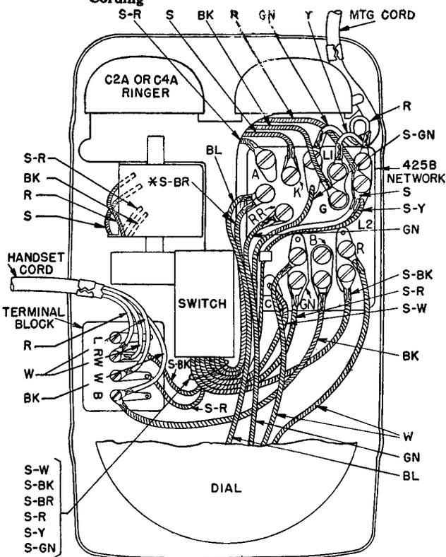
Fig. 17—500C (Manual) and 500D (Dial) Telephone Sets Converted from 500J/K Telephone Sets—Cording
