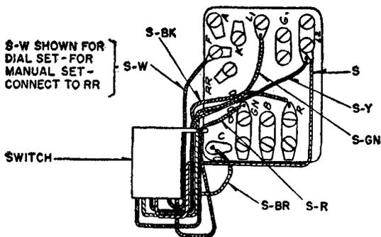
Fig. 10B—501C (Manual) and 501D (Dial) Telephone Sets with C4A Ringer—Switch Detail
