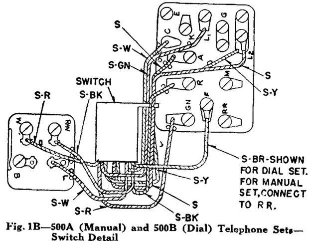
**Fig. 1B—500A (Manual) and 500B (Dial) Telephone Sets—Switch Detail**
