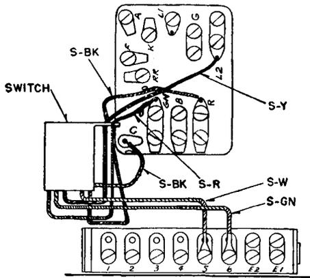
Fig. 6B—500L (Manual) and 500M (Dial) Telephone Sets—Switch Detail
