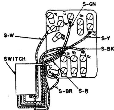
Fig. 11B—501F (Dial) Telephone Set—Switch Detail
