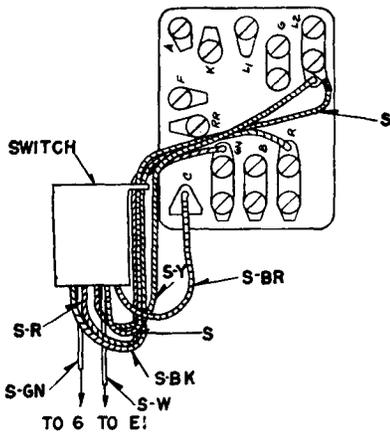
Fig. 4B—500H (Dial) Telephone Set—Switch Detail
