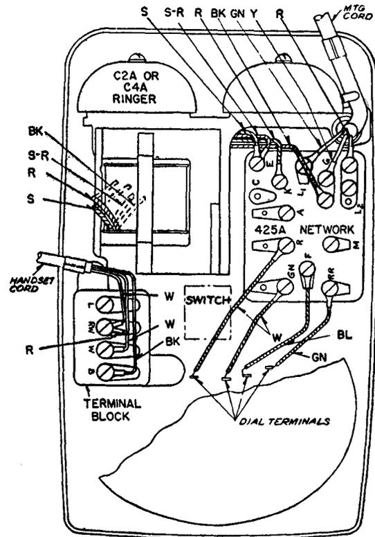
Fig. 5A—500J (Manual) and 500K (Dial) Telephone Sets—Cording
