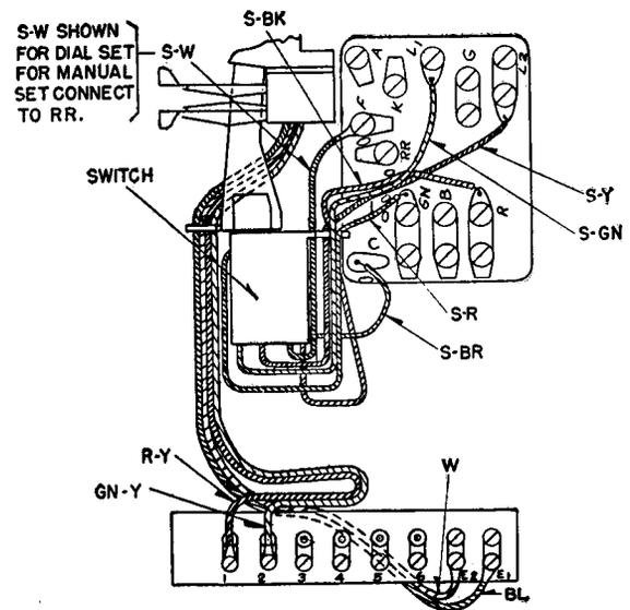
Fig. 16B—511A (Manual) and 511B (Dial) Telephone Set—Switch Detail
