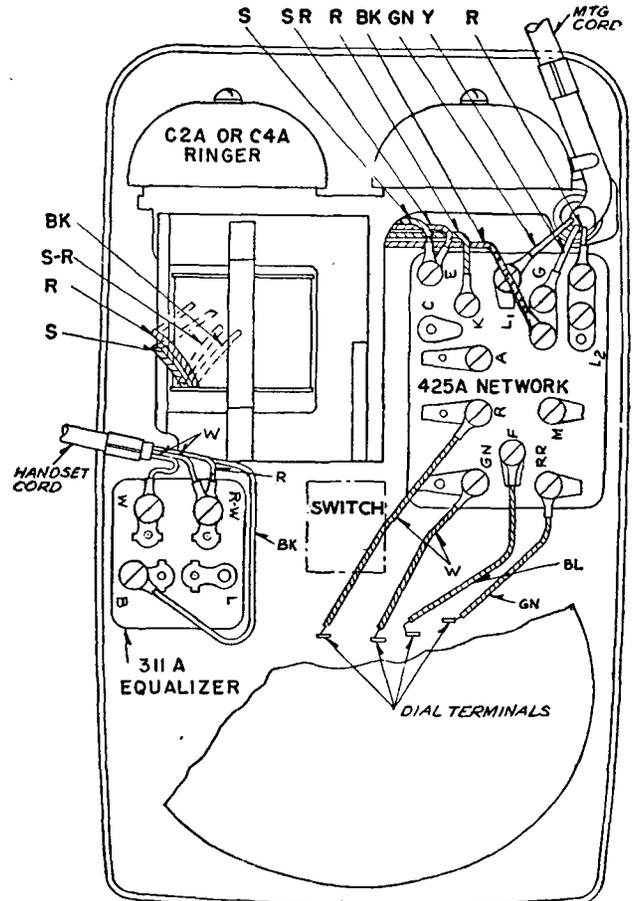
**Fig. 1A—500A (Manual) and 500B (Dial) Telephone Sets—Cording**
