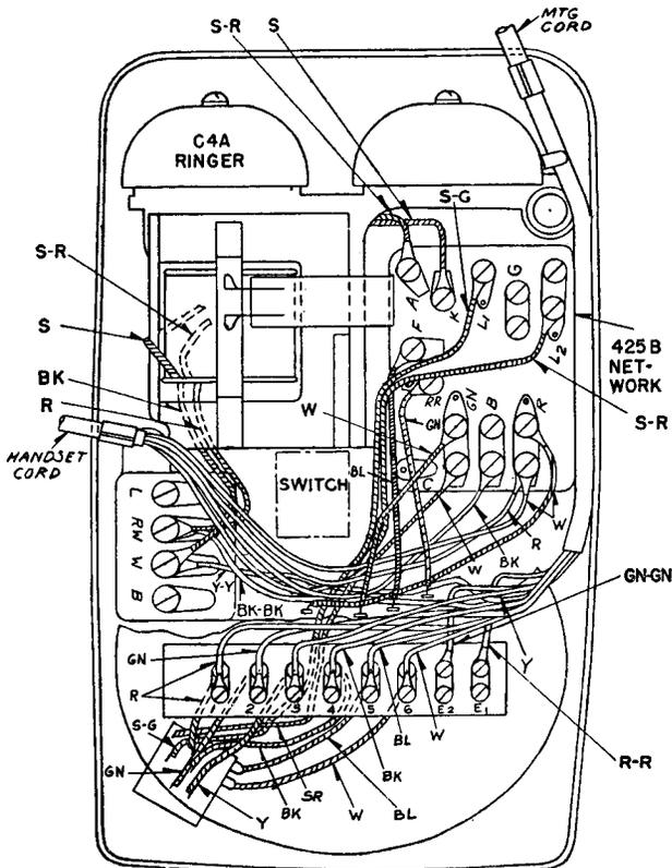
Fig. 16A—511A (Manual) and 511B (Dial) Telephone Set—Cording
