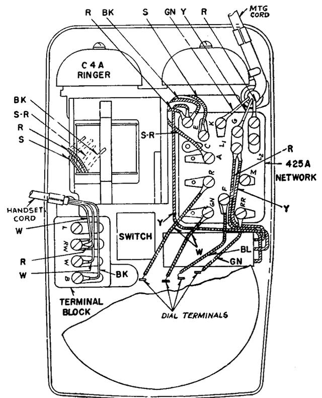
Fig. 13A—501J (Manual) and 501K (Dial) Telephone Sets with C4A Ringer—Cording
