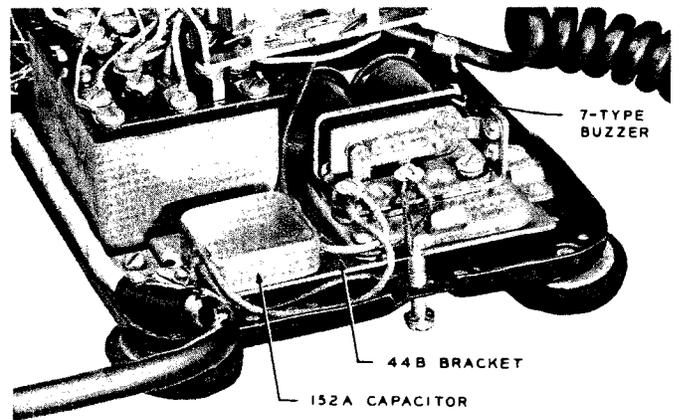
Fig. 9 — 7-Type Buzzer and 44-Type Bracket
