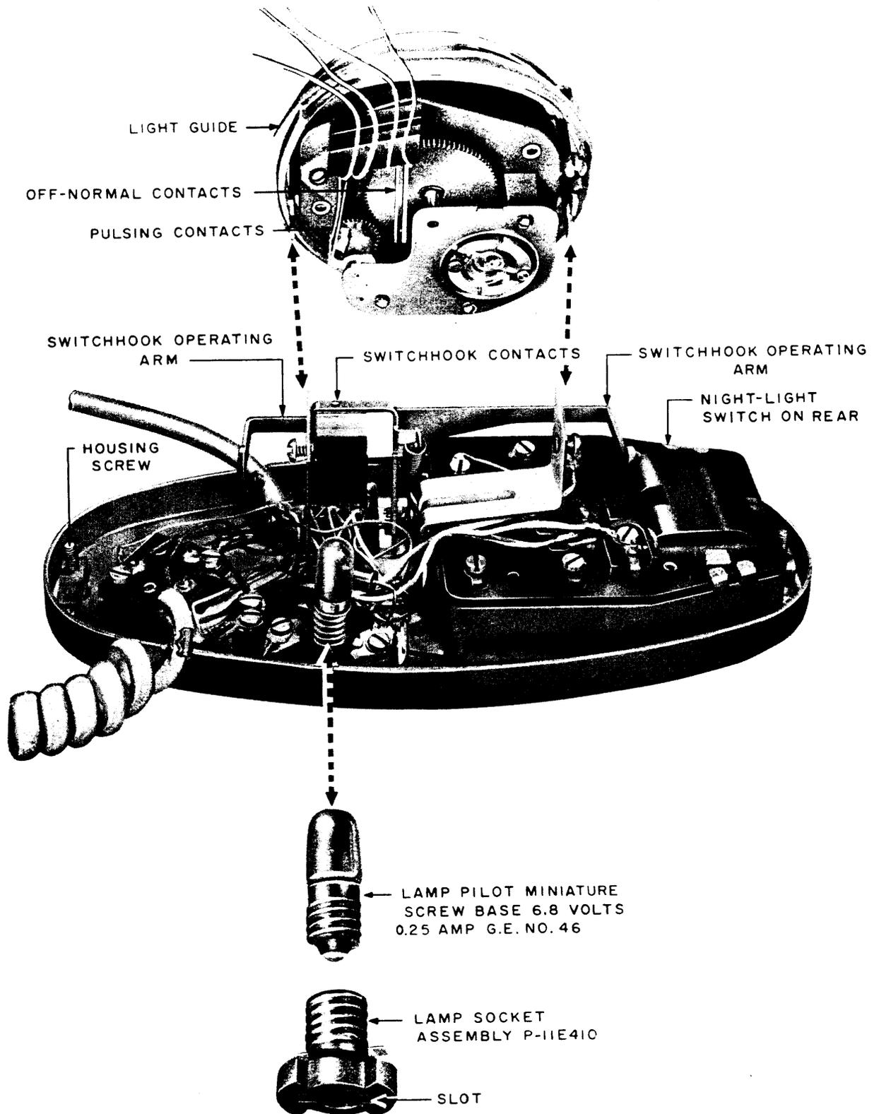
Fig. 8 — 701B Telephone Set with Dial and Lamp Socket Removed
