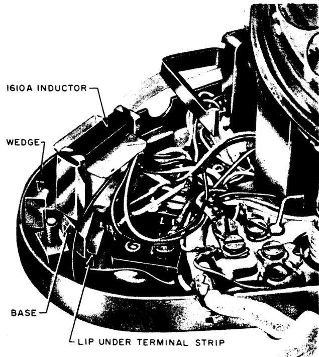
Fig. 6 - 1610A Inductor Installed in 701B Telephone Set
