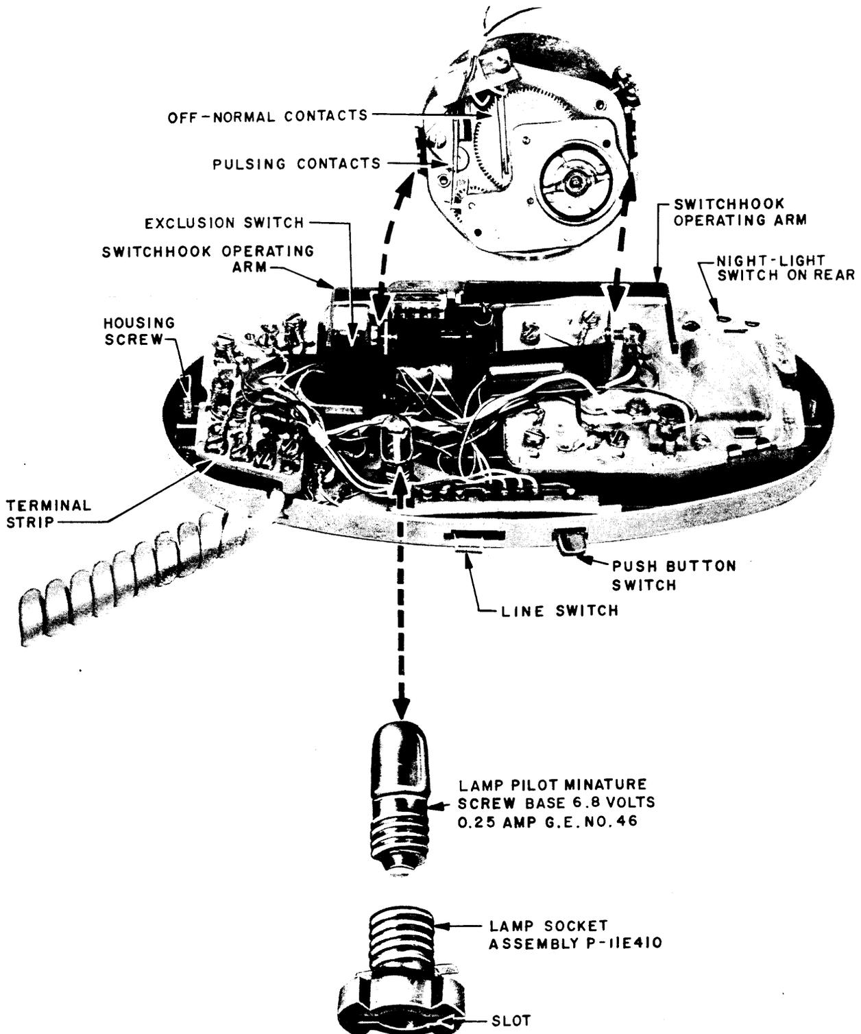
Fig. 9 - 711B Telephone Set with Dial and Socket Removed
