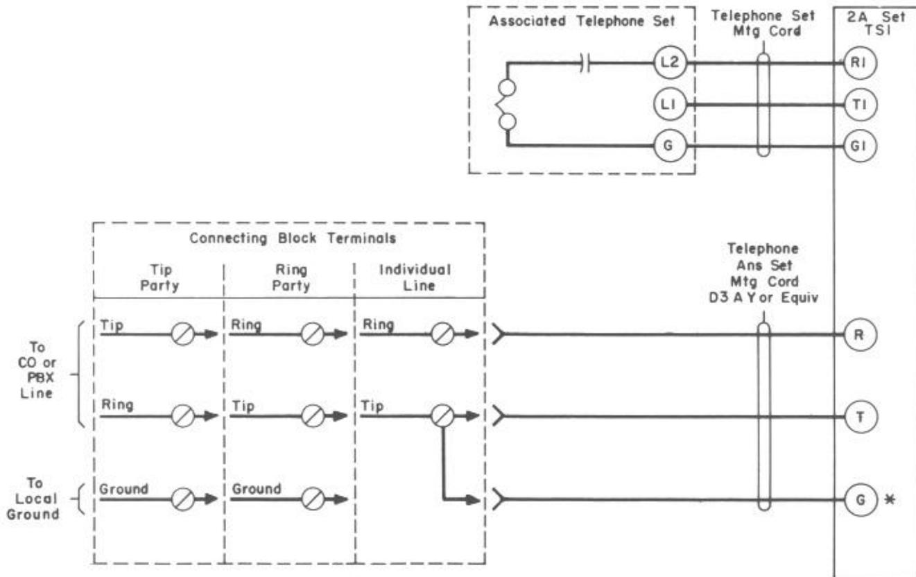
Fig. 1 - 2A Telephone Answering Set, Station Connections for Individual Line, 2-Party Selective, Flat or Message Rate, Manual or Dial
