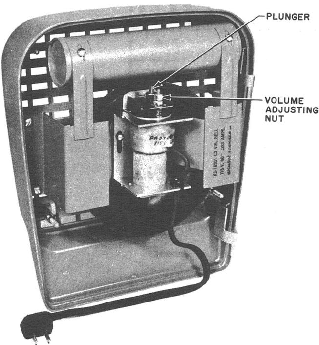
◀ **List 3 Bell, Vibrating** (Fig. 4) — An ac-operated vibrating bell signal which employs a 580-cycle, resonated, 6-inch steel gong. A volume adjustment control is provided which has a range of about 10 db. Maximum volume output is 100 db.
