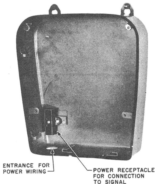
**List 10 Back Box** (Fig. 14) — Is intended for outdoor, dual-potential use and is equipped with a power receptacle to which a 3-conductor, 4-foot cord is connected. The cord has a 3-blade plug and a weatherproof cap for connection to a weatherproof commercial power outlet. Insertion of plug grounds the signal housing.
