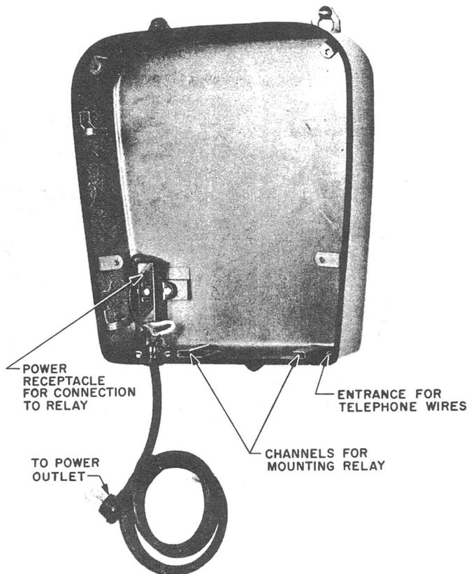
◀ **List 8 Back Box** (Fig. 12)—Is intended for indoor, dual-potential use and is equipped with a power receptacle to which a 2-conductor, 4-foot cord is connected. The cord has a 2-blade plug to connect to the commercial power outlet.
