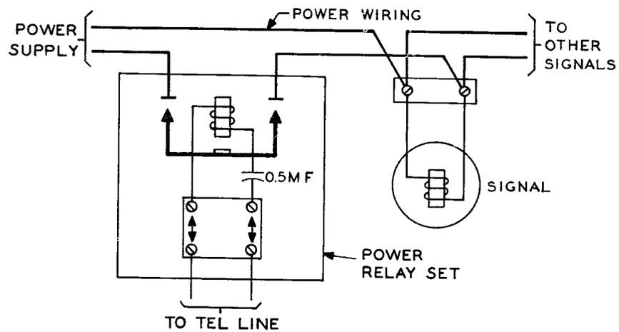
**Fig. 6 – KS-7340, or Equivalent, Power Relay Set Connections**
