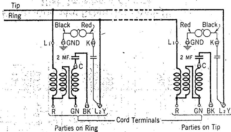
**Fig. 2—Divided Code Ringing Anti-Sidetone Stations—High Impedance Ringers**
