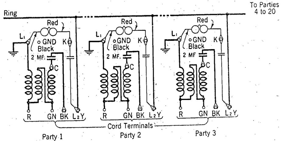
**Fig. 3—Grounded Return Line Anti-Sidetone Stations—
