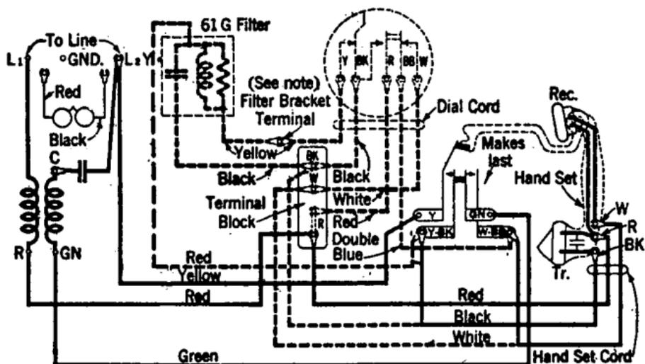
Note: If filter is not provided connect yellow lead from Y of dial to Y-BK mounting contact instead of filter bracket terminal.
