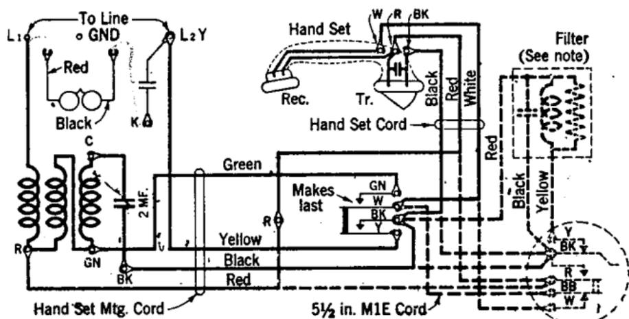
Note: If filter is not provided connect BK mounting contact to Y of dial with 5 1/2 in. M1E cord
