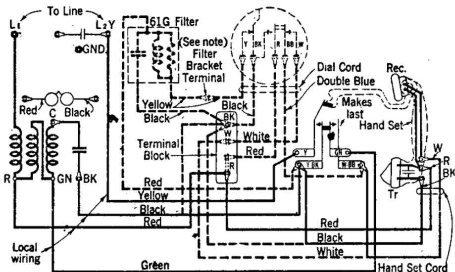
Note: If filter is not provided connect yellow lead from dial to Y-BK mounting contact instead of to filter bracket terminal.
