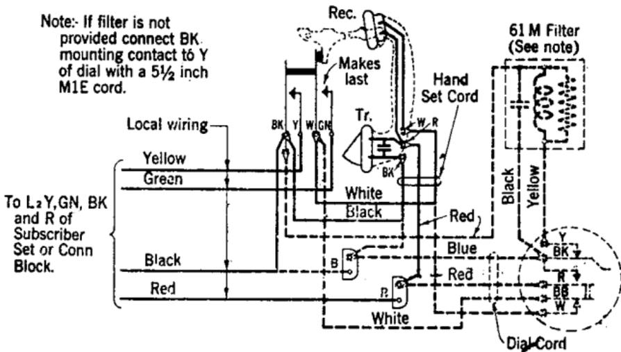
Fig. 5 - 211 Type Hand Telephone Sets
