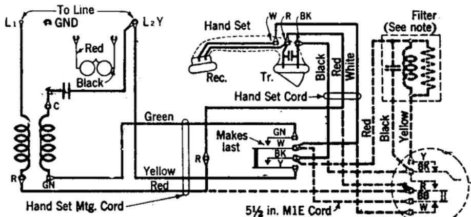
Note: If filter is not provided connect BK mounting contact to Y of dial with 5 1/2 in. M1E cord.
