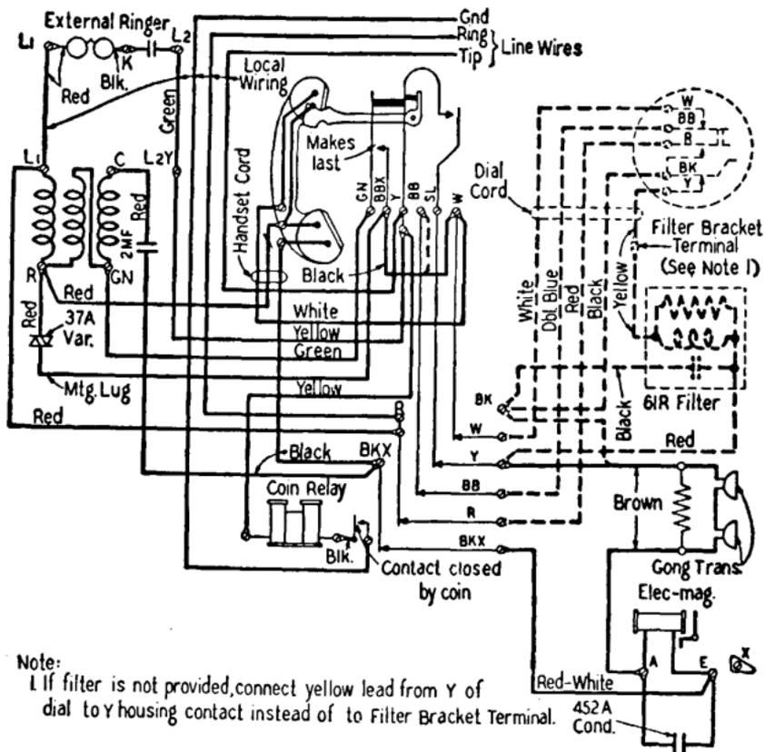
**Fig. 10—191C, E, or G Coin Collector with 101A Ind. Coil**
