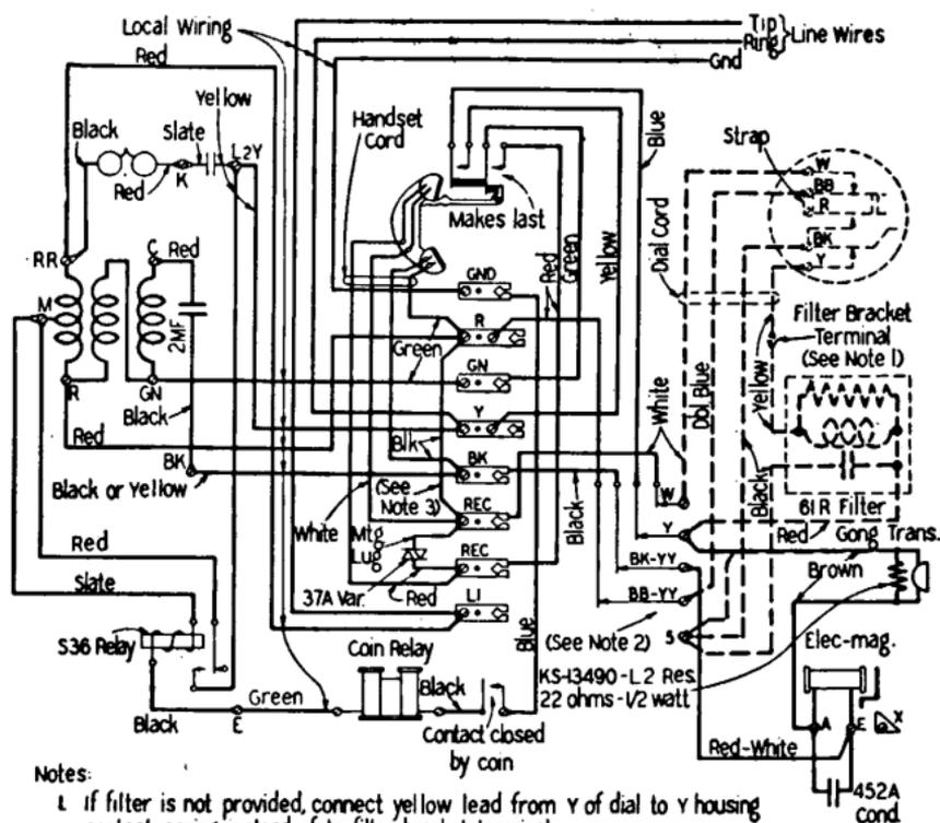
1. If filter is not provided, connect yellow lead from Y of dial to Y housing contact spring, instead of to filter bracket terminal.
