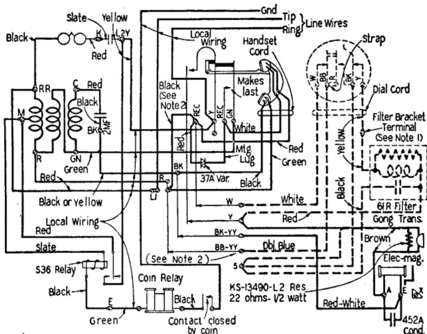
**Fig. 19—176C, E, or G Coin Collector with 634CG or CH Sub. Set**
