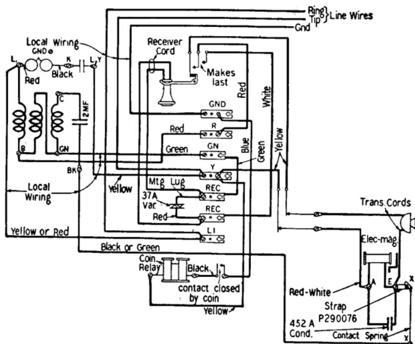
Fig. 1—55AC Coin Collector
