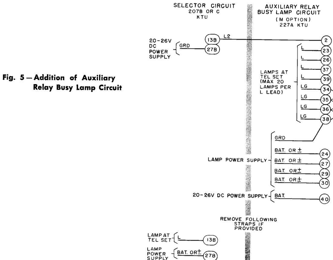
**Fig. 5 – Addition of Auxiliary Relay Busy Lamp Circuit**
