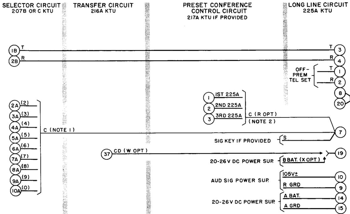
**Note 1:** C leads that operate long line circuits must connect through the first bank of the selector when the selector only arrangement is used. Off-premise stations must be assigned single-digit codes.
