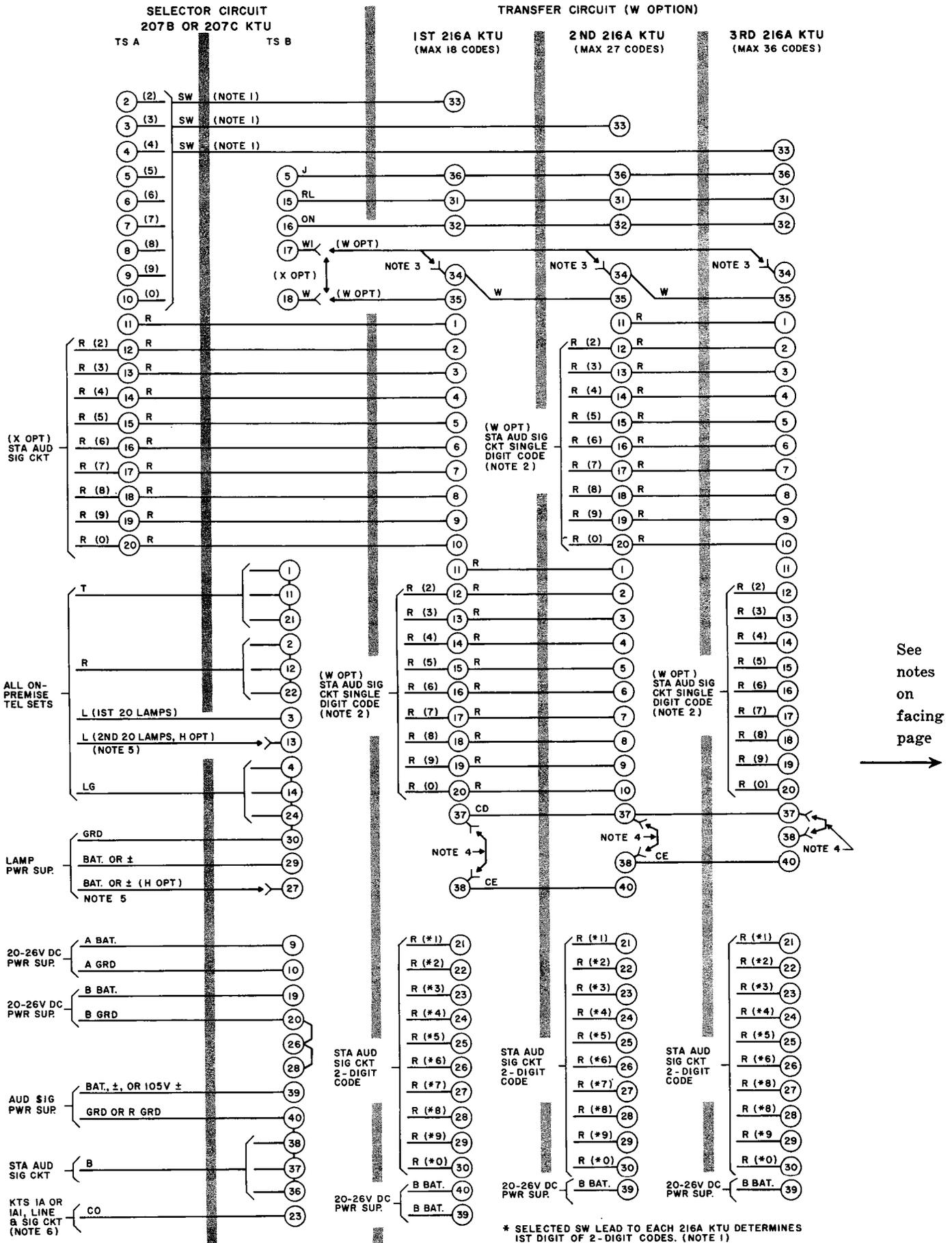
Fig. 1 — Selector Circuit Connections to Transfer Circuit
