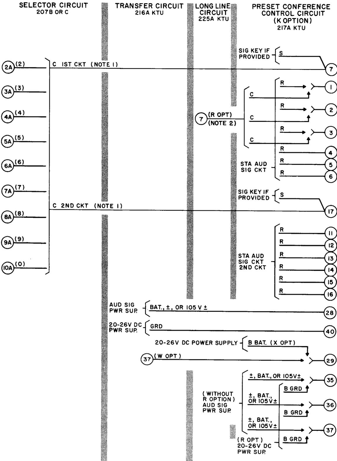
**Note 1:** C leads that operate preset conference circuits must connect through the first bank of the selector when the selector only arrangement is used. Single digit codes must be assigned to operate preset conference circuits.
