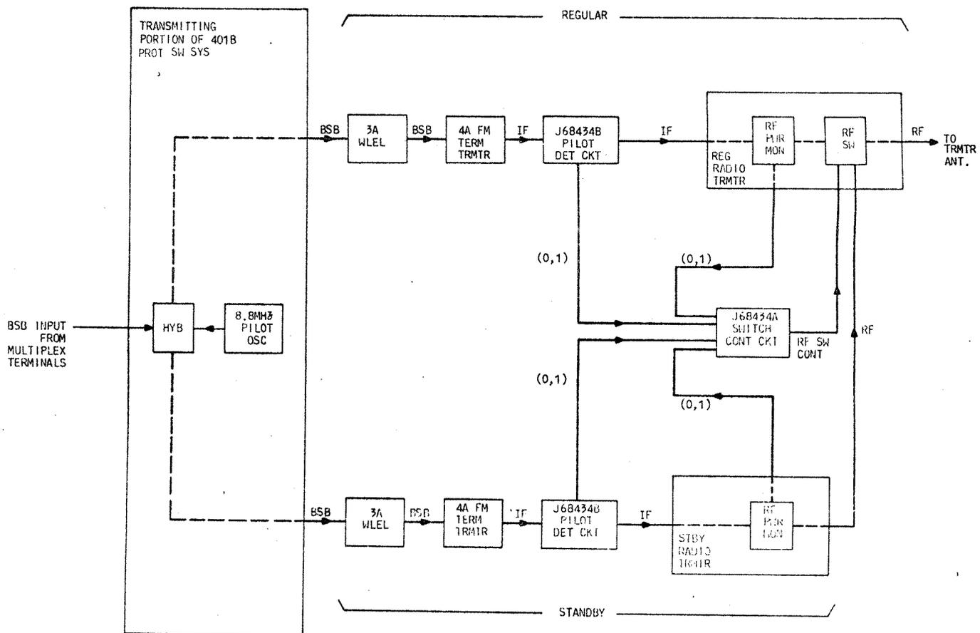
CD Fig. 3 - Typical Transmitting Terminal Arrangement for HS or HS/SD Systems
