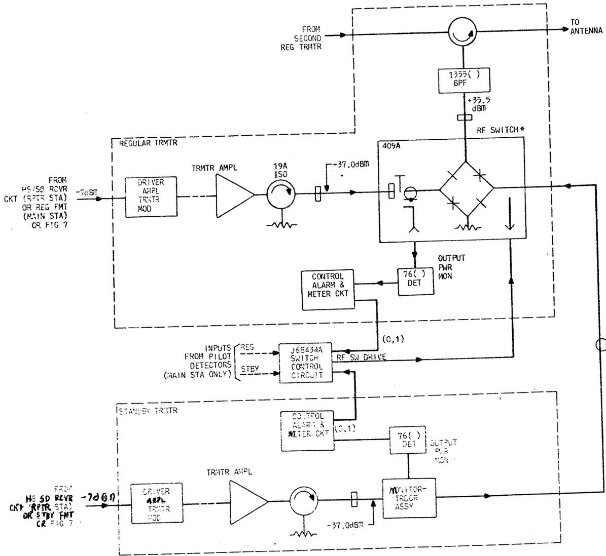
\* THIS ARRANGEMENT EMPLOYS THE 409A DIODE TYPE SWITCH IN PLACE OF THE ELECTROMECHANICAL COAXIAL SWITCH AS SHOWN IN FIGS. 2 AND 3.
