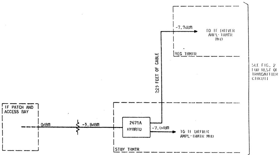
CD Fig. 7 - Connection of HS Transmitter to IF Patch and Access Bay
