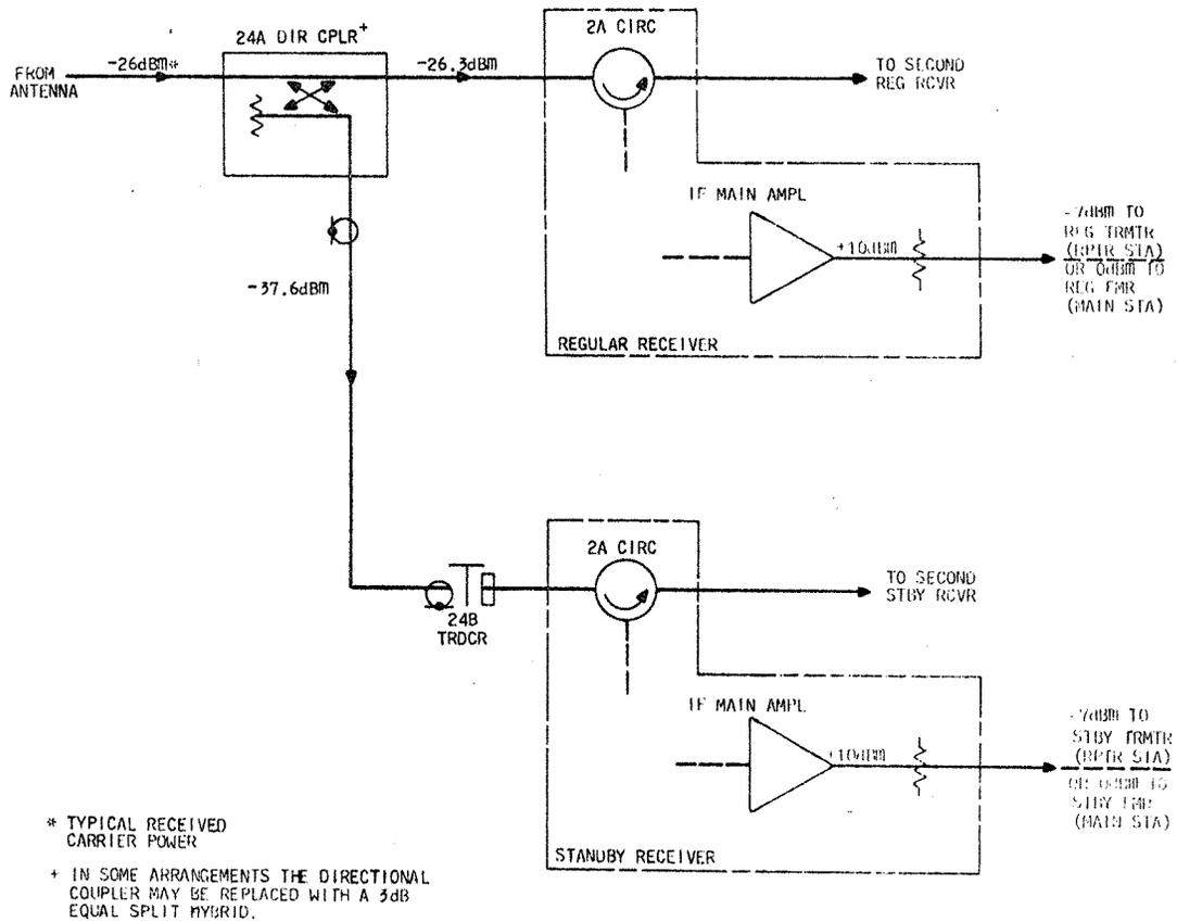
CD Fig. 1 - Receiver Circuit for Hot Standby Only Applications
