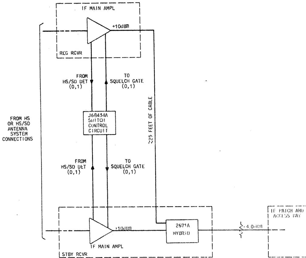
CD Fig. 6 - Connection for HS or HS/SD Receiver Circuit to Patch and Access Bay
