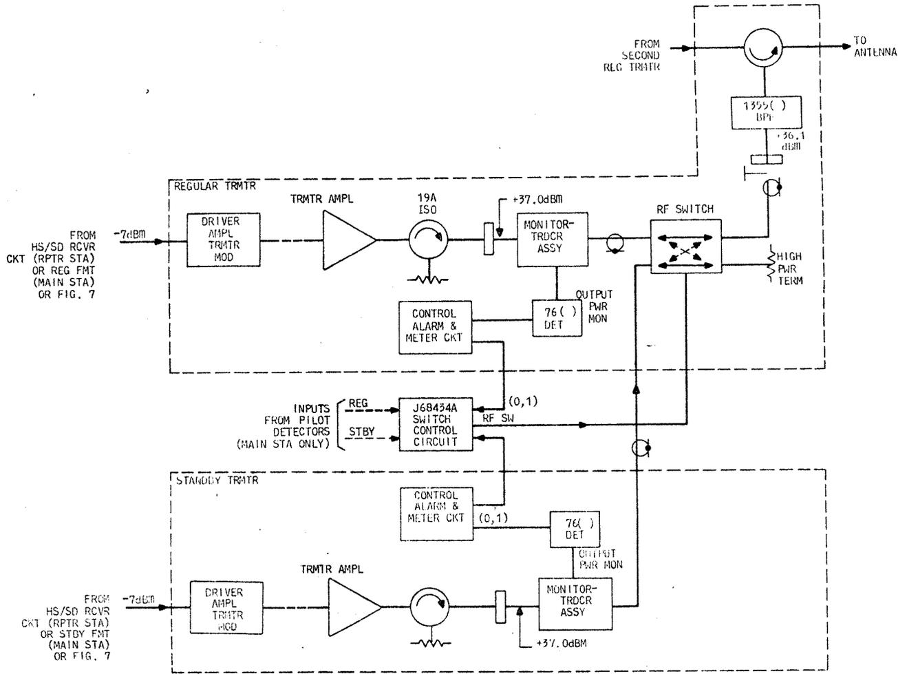
CD Fig. 2 - Transmitter Circuit for HS or HS/SD Applications
