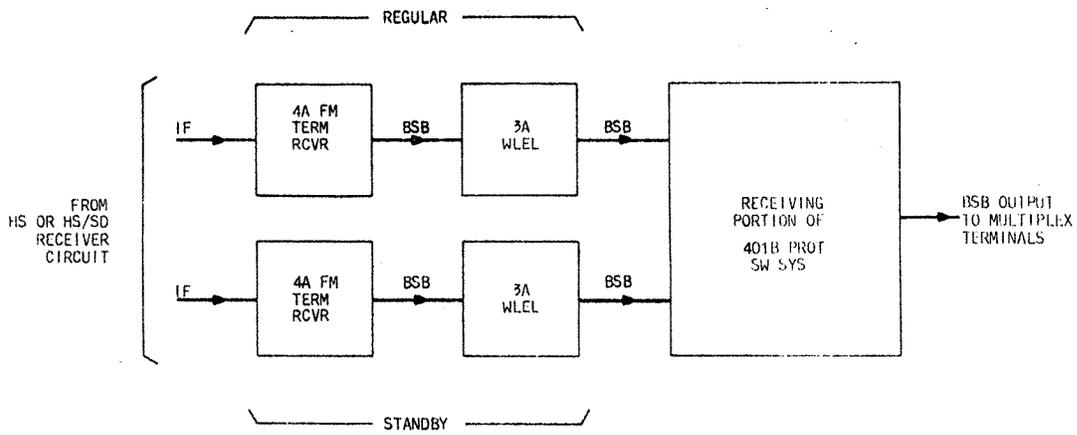
CD Fig. 4 - Typical Receiving Terminal Arrangement for HS or HS/SD Systems
