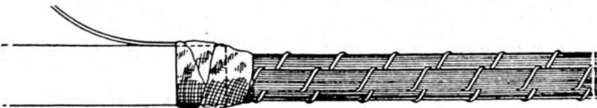
5.05 Straight Splice: Apply one half-lapped layer of muslin over the splice, extending the muslin about 1 inch beyond the DR tape at each end as illustrated. Solder the bonds from each side on top of the splice as indicated. Then clean 2 inches of sheath at each end and coat the cleaned area with C cement.
