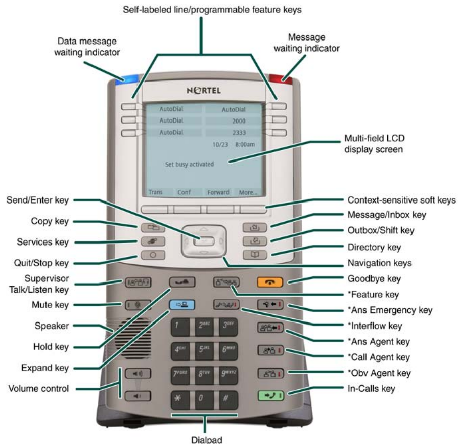
Figure 59 IP Phone 1150E Supervisor key configuration
