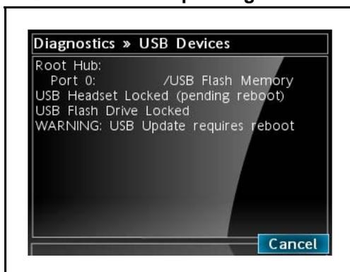
Figure 110 "USB devices - lock pending" (page 628) above shows an 1165E phone with a USB Flash Drive connected and enumerated. The USB Headset and USB Flash Drive device types have been locked in the USB Locks menu but the USB Headset lock is waiting on a reboot of the phone for the lock to take effect. Once the phone is rebooted, the Warning and "(pending reboot)" message will disappear and the USB Headset device is just shown as locked.
