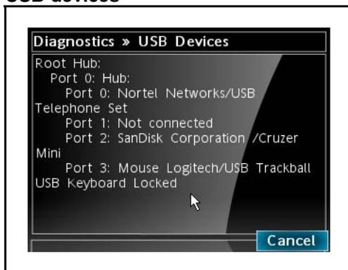
Figure 109 "USB devices" (page 628) above shows an 1165E phone with a Nortel USB Headset adapter, USB Flash Drive and USB trackball connected and enumerated. The text "USB Keyboard Locked" shows the USB Keyboard device type has been locked in the USB Locks menu.
