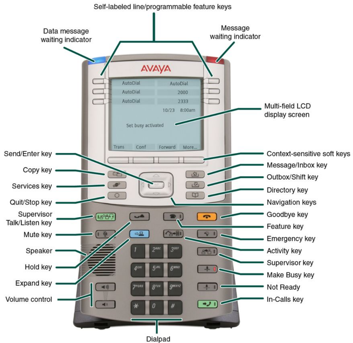
Figure 50: Avaya 1150E IP Deskphone Supervisor key configuration
