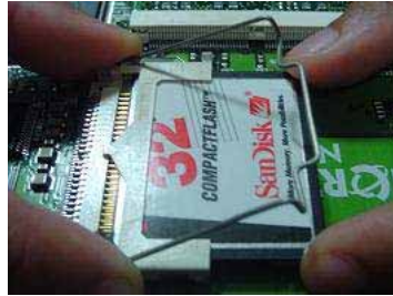
Figure 13 CFlash card with metal clip up
