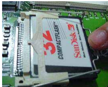
Figure 14 CFlash card with metal clip down
