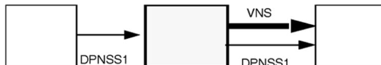
Figure 126: DPNSS1/VNS with DPNSS1 node
