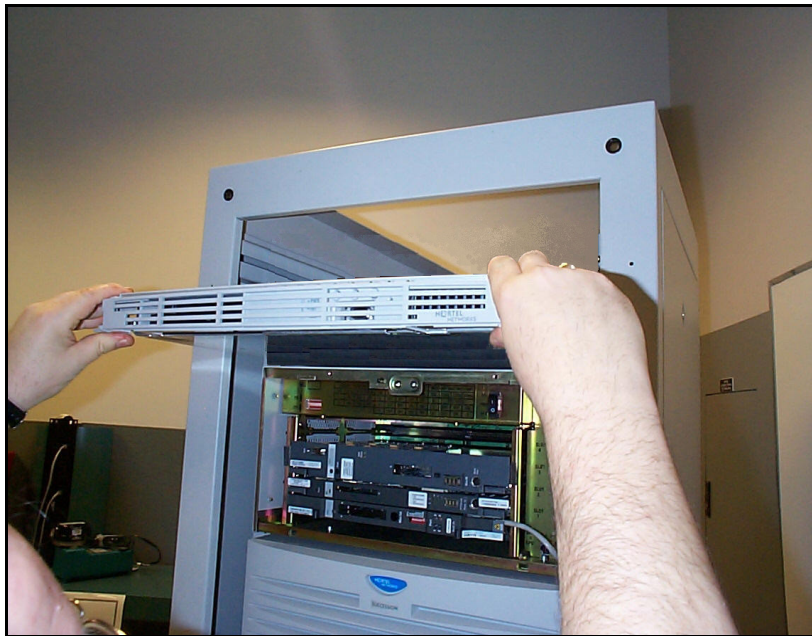
Figure 50 Rack-mounting the ISP1100 Signaling Server
