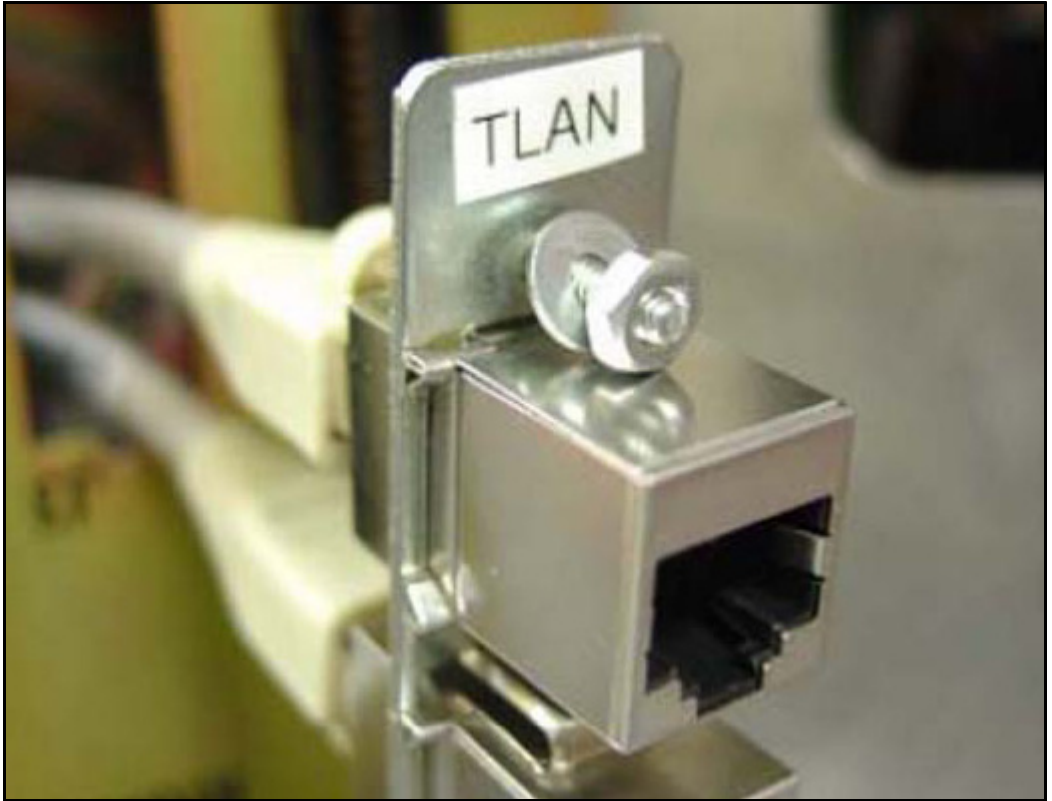
Figure 30 TLAN connection on Ethernet port coupler
