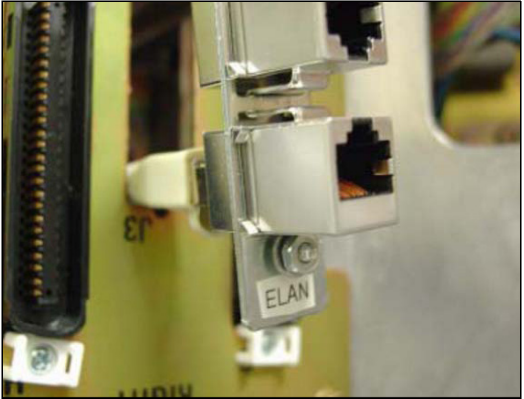
Figure 28 ELAN connection on Ethernet port coupler
