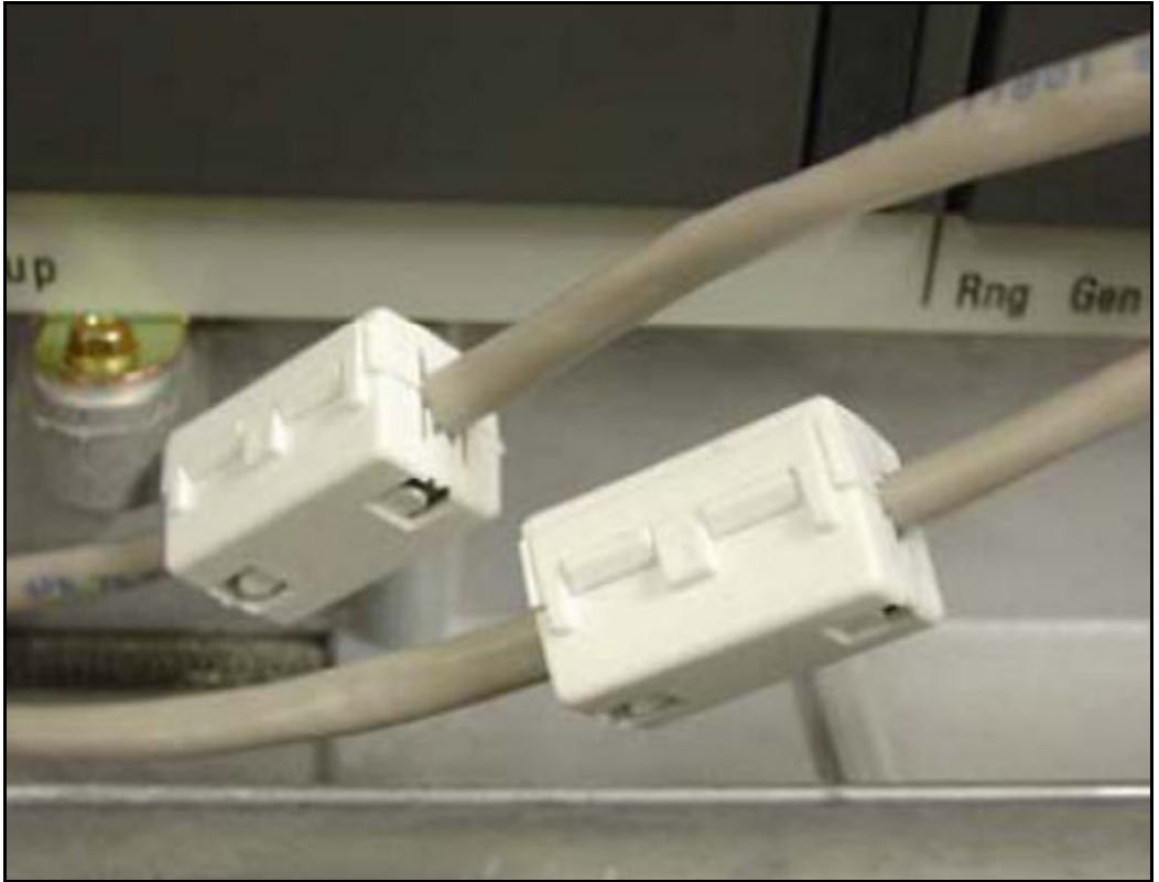
Figure 32 Attached Ethernet patch cable ferrite beads
