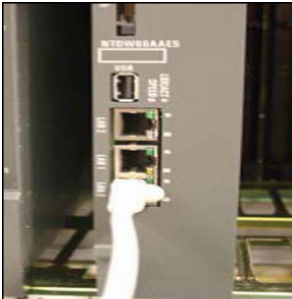
Figure 27 ELAN connection on faceplate
