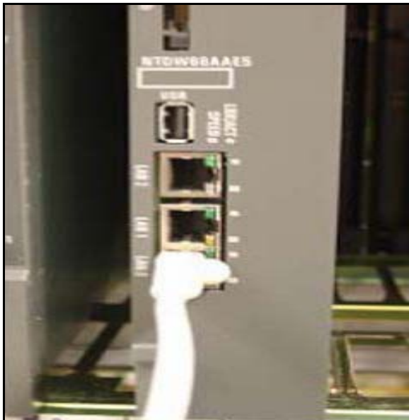
Figure 29 ELAN connection on the CP PM faceplate
