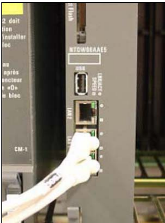
Figure 31 TLAN connection on the CP PM faceplate
