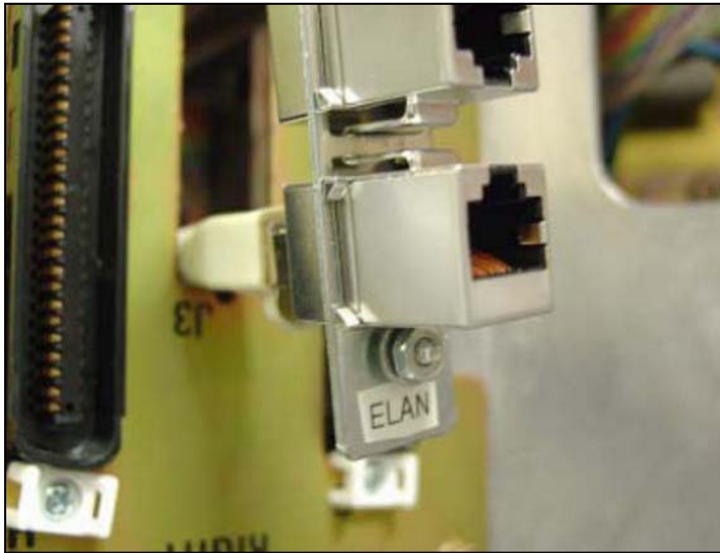
Figure 30 ELAN connection on Ethernet port coupler
