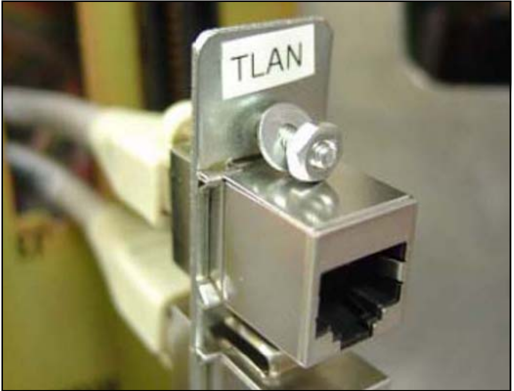
Figure 32 TLAN connection on Ethernet port coupler
