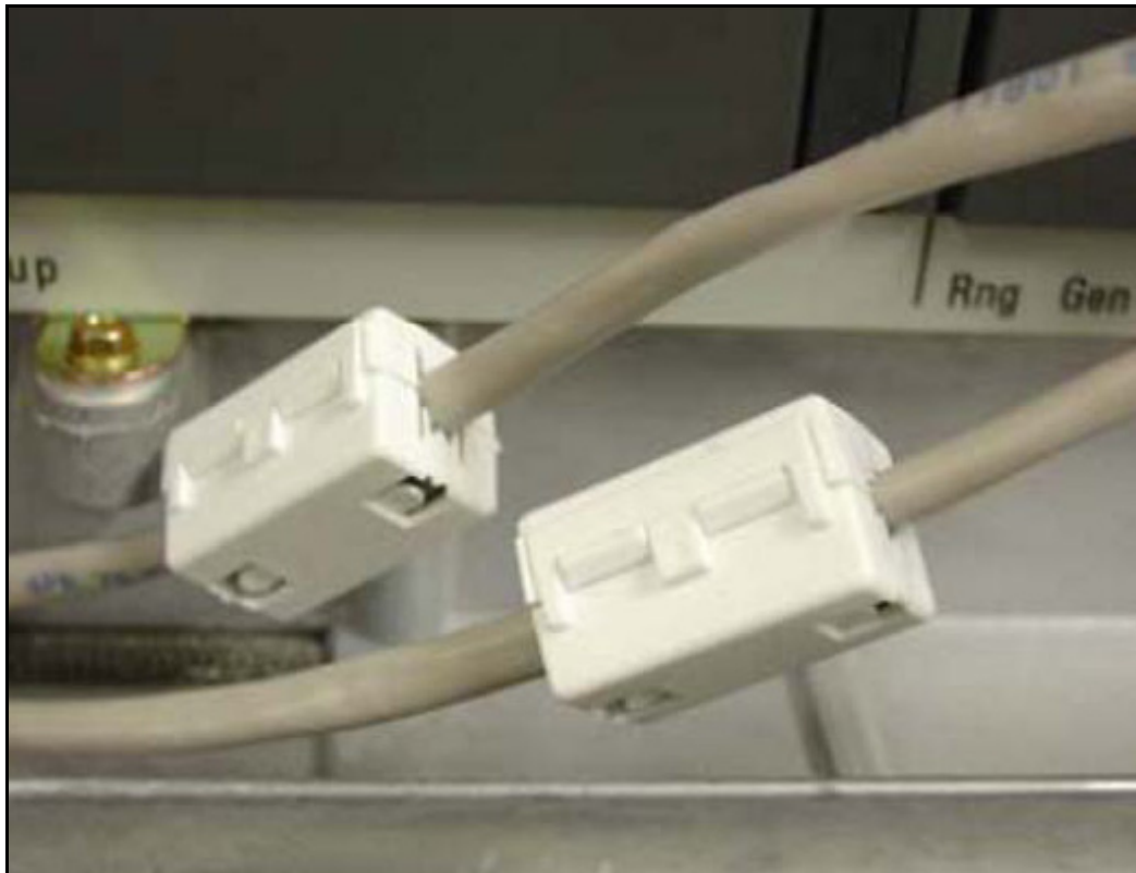
Figure 54 Attached Ethernet patch cable ferrite beads
