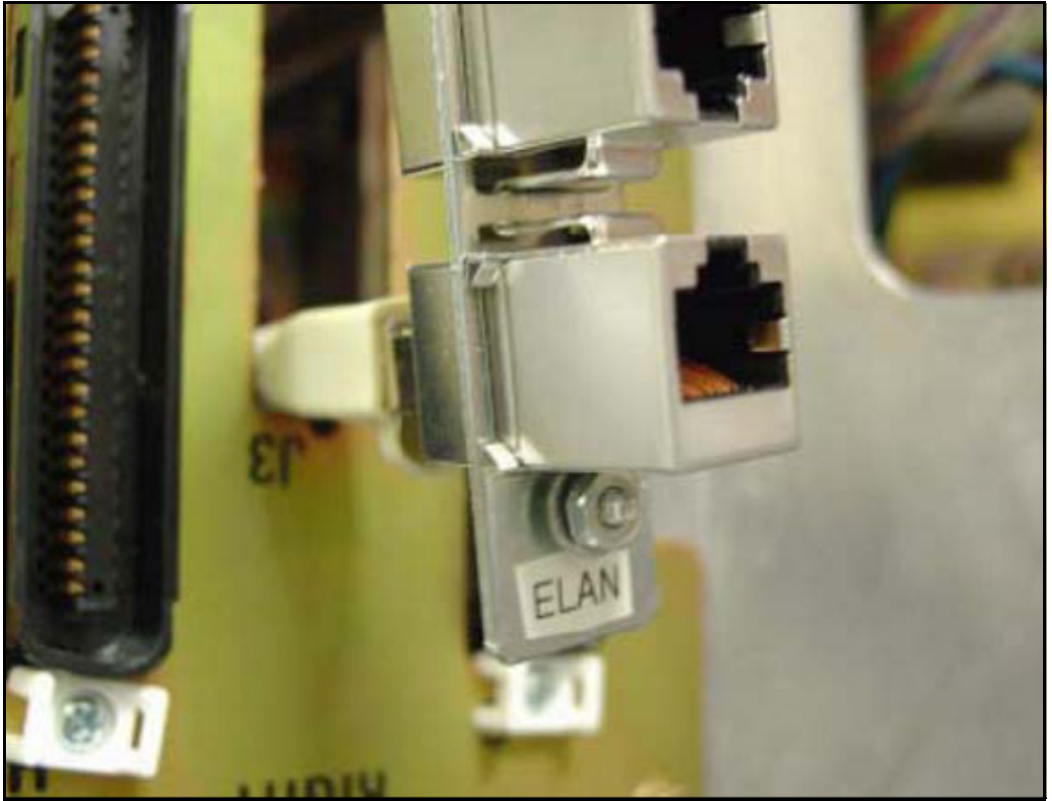
Figure 18 ELAN connection on Ethernet port coupler
