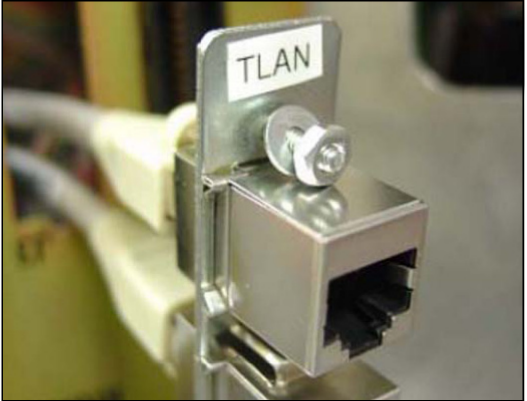
Figure 37 TLAN connection on Ethernet port coupler
