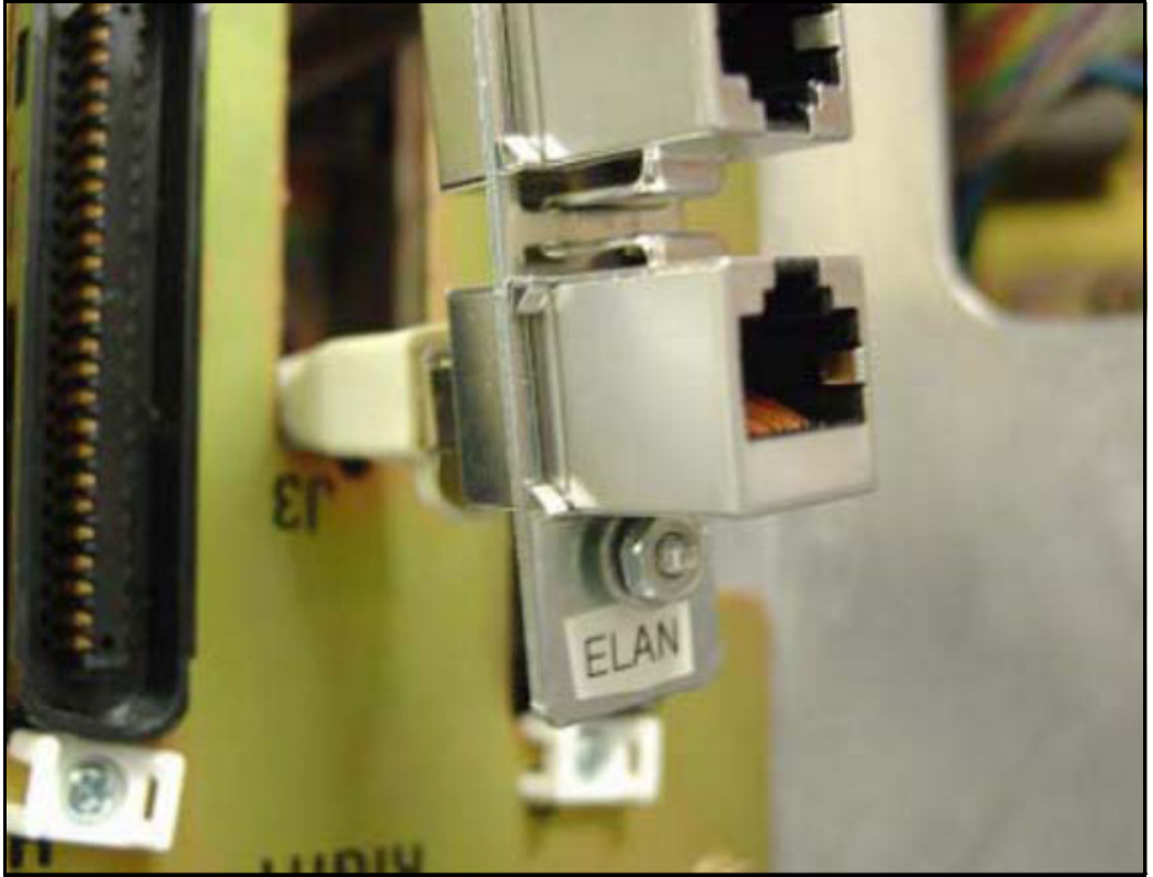
Figure 35 ELAN connection on Ethernet port coupler
