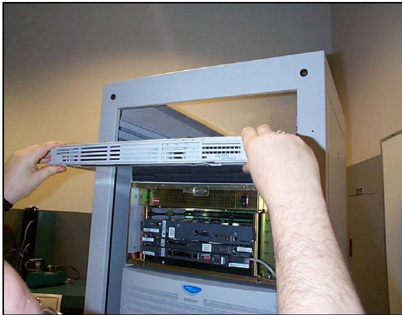
Figure 57 Rack-mounting the ISP1100 Signaling Server
