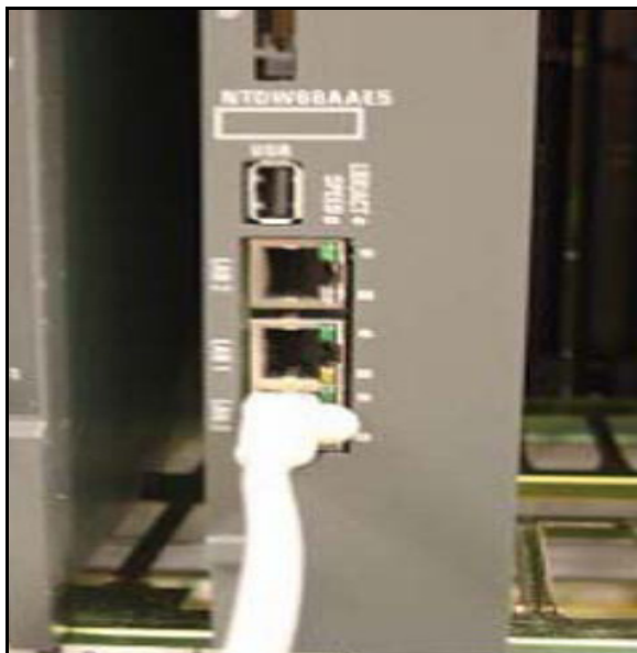
Figure 29 ELAN connection on faceplate
