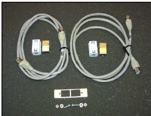
NTDW69AAE5 Cabling Kit contents
