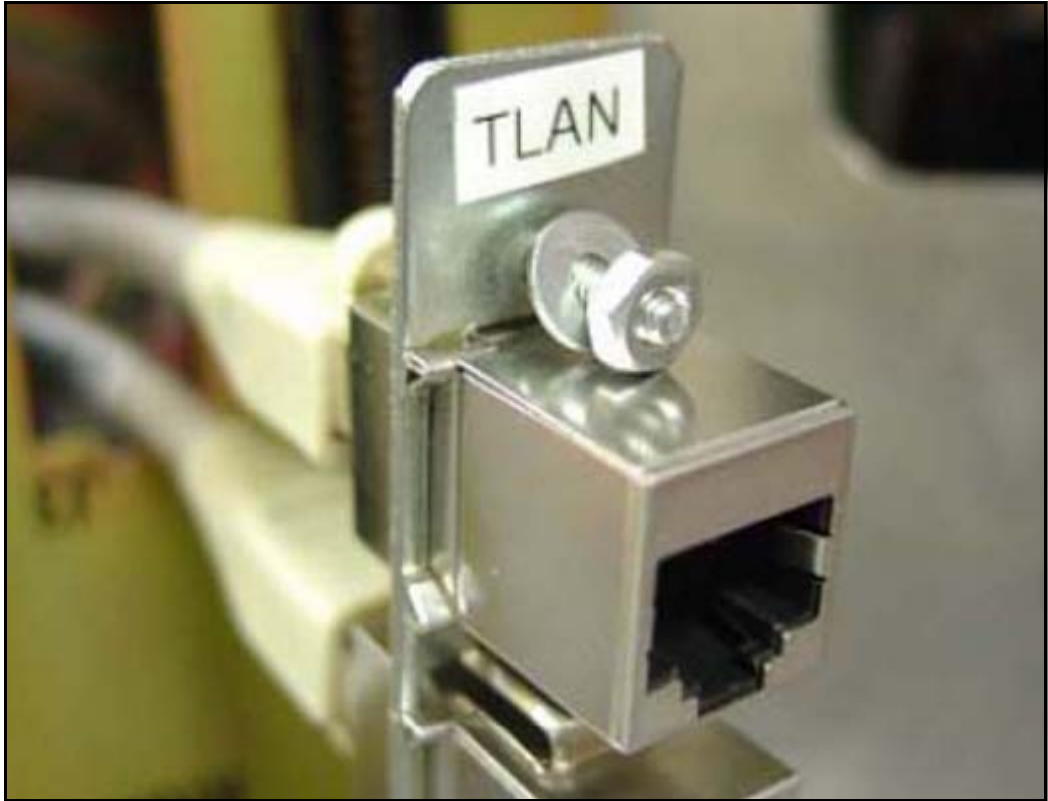
Figure 51 TLAN connection on Ethernet port coupler
