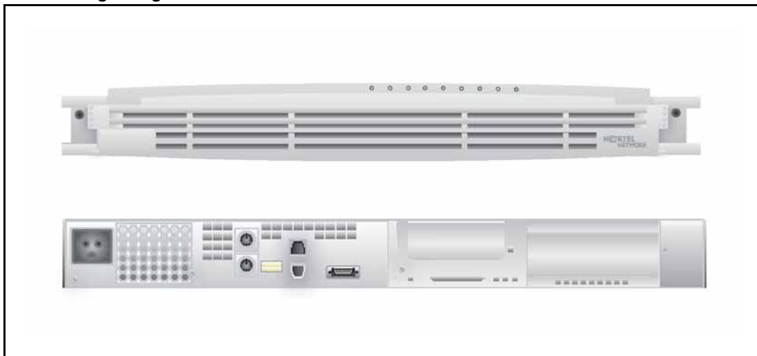
Figure 22 ISP1100 Signaling Server front and rear
